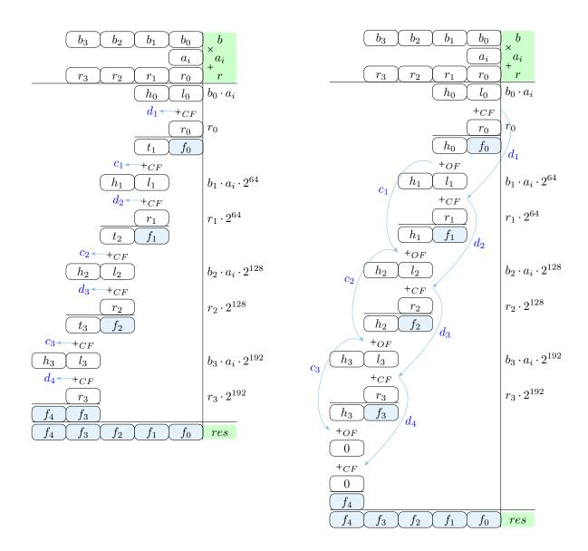
Figure  $3.4 - 256 \times 64$ -bit multiplication with a 256-bit accumulator. On the left, using the ADC and ADD instructions, and on the right, using the ADX and MULX instructions. The ADC and ADD instructions compute addition with and without a carry, respectively, and share the same carry flag. The ADX instruction set supports two additions, ADOX and ADCX, with independent carry flags, which allows computing multiplication with two parallel carry chains.
