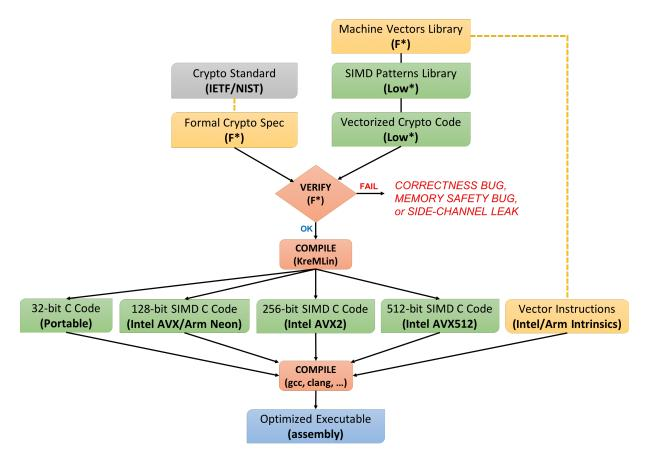
Figure 4.1 – HACL×N programming and verification workflow. We write SIMD cryptographic code in Low\* [108] and prove it memory-safe, secret independent, and functionally correct with respect to a high-level formal specification in F\* [118], before compiling it to target-specific C code linked with compiler intrinsics. (Code components in green are verified; those in yellow are trusted and carefully tested.)
