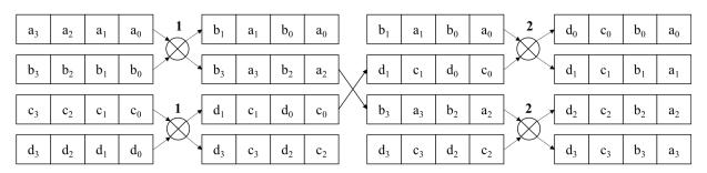
Figure 4.5 – Transposing a  $4 \times 4$  vectorized state. Each pair of vectors is interleaved element by element, then each alternate pair is interleaved 2 at a time. Transposing a  $n \times n$  vectorized matrix needs  $n \log_2(n)$  interleavings.
