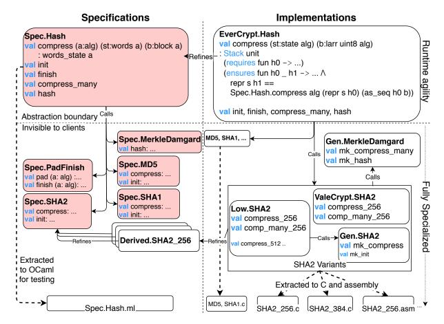
Figure 3.2 – The modular structure of EverCrypt (illustrated on hashing algorithms)
