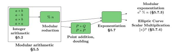
Figure 5.1 – High-level specification for Modular Exponentiation and Elliptic Curve Scalar Multiplication.
