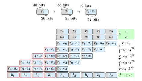
Then, we can perform reduction modulo  $p = 2^{130} - 5$  of the product  $b = r \cdot a$  by multiplying  $b_5$  by 5 and adding the product to  $b_0$ ,  $b_6 \cdot 5$  to  $b_1$  and so on:
