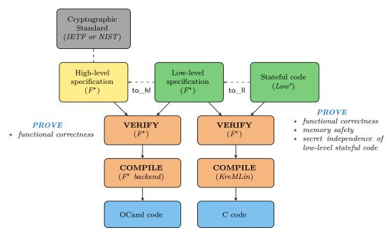
Figure 2.1 – HACL\* programming and verification workflow.
