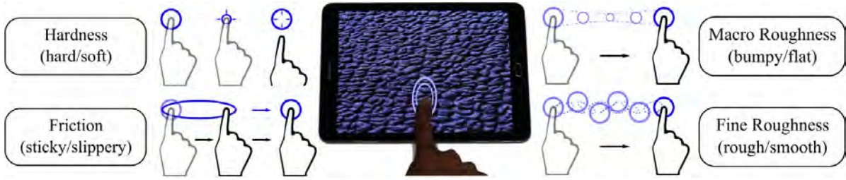
Figure 8: Touchy is a co-localized cursor for tactile displays that deforms and/or moves to evoke a variety of haptic properties, covering four different perceptual dimensions: fine roughness, macro roughness, hardness, and friction.
