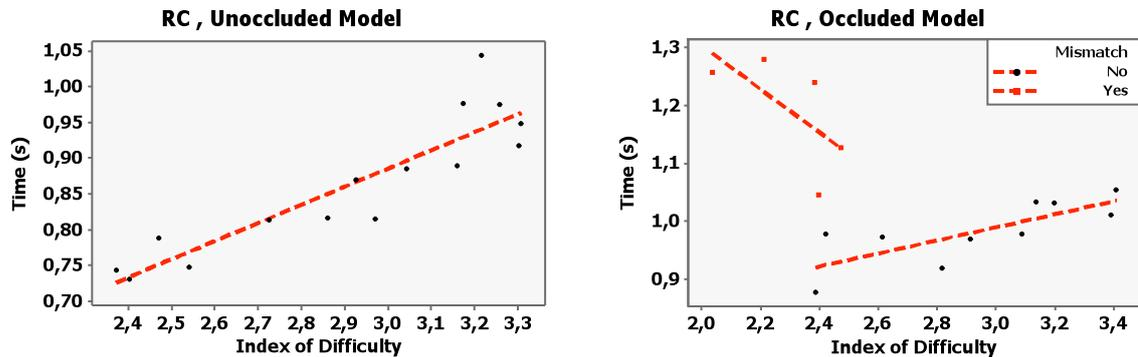
Figure 6: Scatterplot of mean object selection time vs index of difficulty for two selection tasks. (Left) All virtual objects did not exhibit eye-hand visibility mismatch ( $r = 0.898$ ). (Right) A number of objects exhibited eye-hand visibility mismatch ( $r = 0.755$ , ignoring the objects with mismatch).
