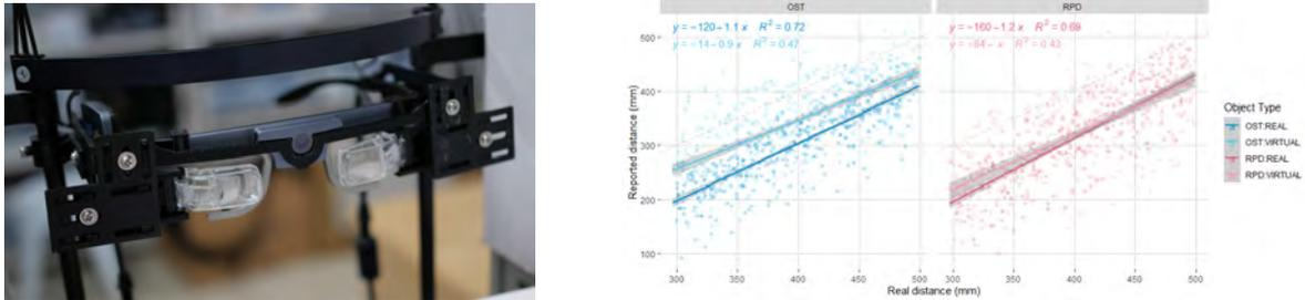
Figure 4: Egocentric distance perception. Left, binocular RPD device used, composed of two QD Laser RETISSA Displays. Each display module had a resolution of  $1024 \times 600$  pixels and an approximate horizontal FoV of  $20^\circ$ . Right, regression analysis of the egocentric distance estimates. The plot shows that in the RPD condition (red) the distance estimates were closer to the real estimates compared to the OST condition (blue).
