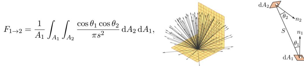
Figure 1.10: View factors formulation without obstacles. Left: integral formula. Middle: uniform hemispherical model. Right: associated configuration where two surface elements are mutually visible.
