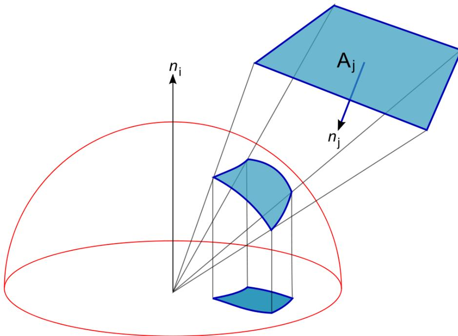
Figure 2.2: Nusselt analog. The view factor between a differential element  $dA_i$  and the element  $A_j$  can be obtained by projecting the element  $A_j$  onto the surface of a unit hemisphere, and then projecting that in turn onto a unit circle around the point of interest in the plane of  $A_j$ . The view factor is then equal to the differential area  $dA_i$  times the proportion of the unit circle covered by this projection. Credits to Jheald.
