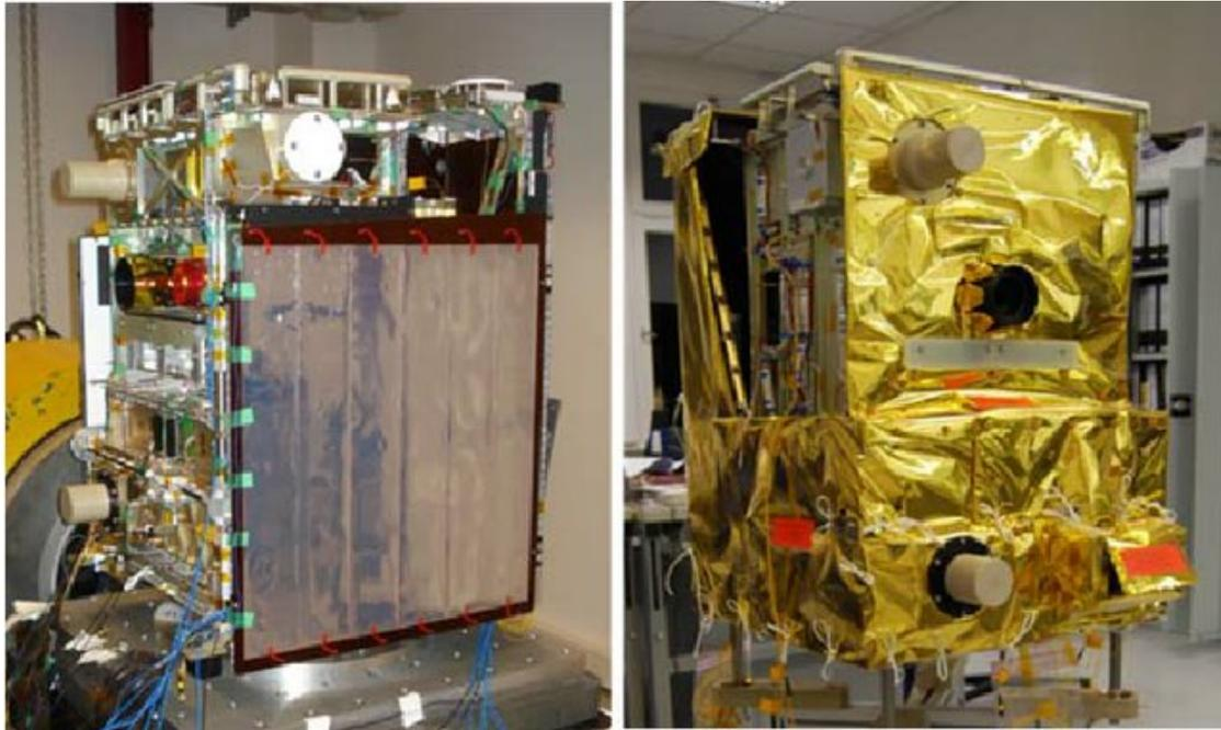
Figure 1.6: Satellite before and after adding Multi-Layer Insulation (MLI) to protect it from extreme radiation. Taken from Fockersperger et al [FLK<sup>+</sup>10].
