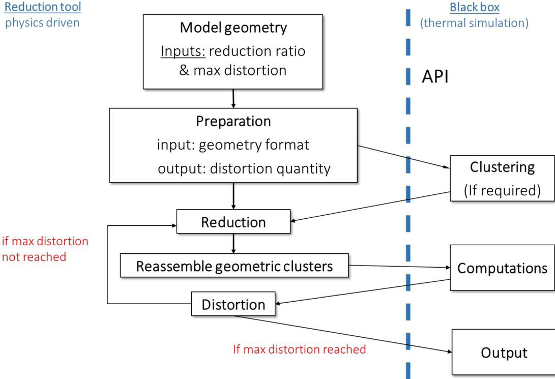
Figure 4.28: Summary of reduction process. Left: mesh reduction. Right: numerical simulation. The reduction and the simulation parts are connected with an API, converting the geometric format to a thermal one from left to right, and returning the maximum error value from right to left. The considered case for this thesis is the radiative thermal simulation, but another numerical simulation could be plugged to the geometric reduction instead.
