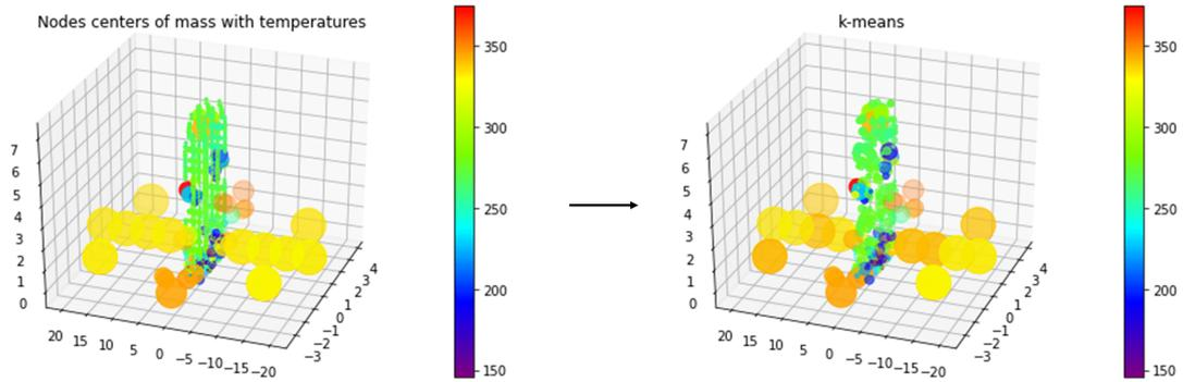
Figure 5.2: K-means clustering algorithm [Llo82] applied to the external part of a satellite (model from DOREA). Reduction from 1400 thermal nodes to 400 clusters with an error of 0.85K degree. K-means take as input the desired number of clusters.
