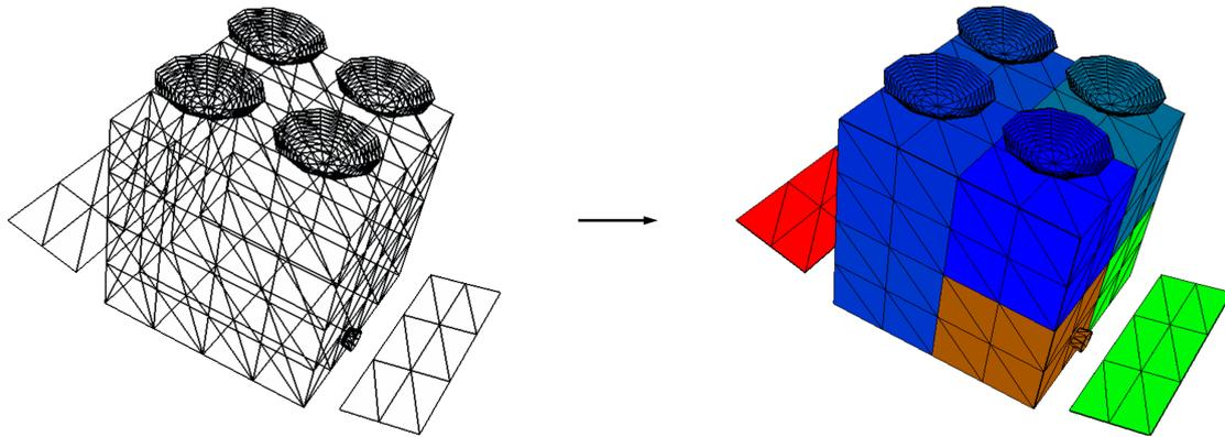
Figure 4.13: Nodal breakdown (i.e., clustering) applied to radiative thermal simulation. Left: geometric input model. Right: nodal breakdown and simulation output. The thermal nodes are depicted.
