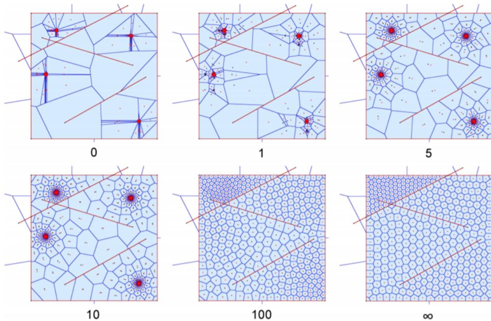
Figure 3.6: 2D centroidal Voronoi tessellation with geometric constraints from Tournois et al [TAD10]. The number of Lloyd iteration is depicted.
