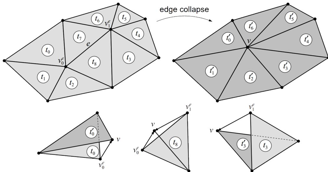
Figure 2.14: Edge collapse operator with tetrahedrons associated to the newly obtained vertex as described by Lindstrom et al [LT98]. Edge  $e$  is collapsed and replaced by vertex  $v$ . Tetrahedrons volumes associated to triangles  $t_0$ ,  $t_3$  and  $t_8$  are depicted.
