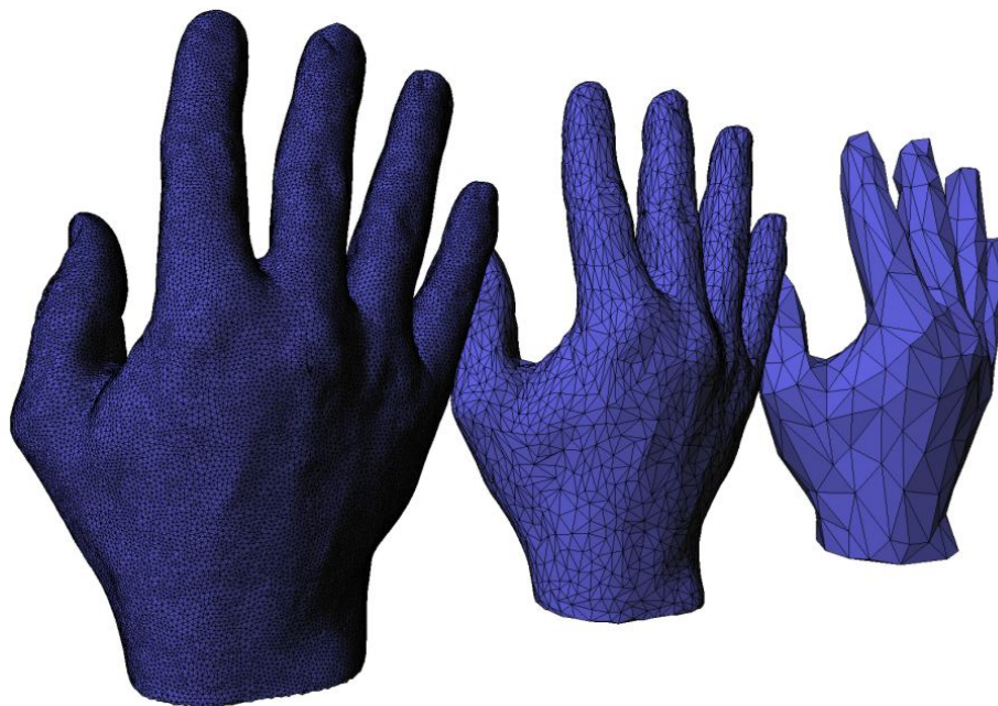
Figure 2.15: Surface mesh simplification from the CGAL library [The20] using Lindstrom-Turk placement and cost strategy.
