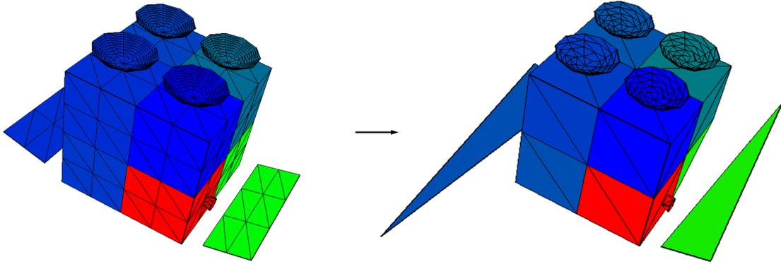
Figure 4.12: Physics-unaware mesh reduction. The maximum distortion tolerance (0.5 degrees) is reached when solar panels are heavily deteriorated, while the antennas can still be reduced (from 1006 to 370 facets).
