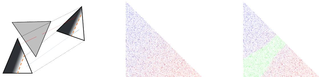
Figure 3.10: Adaptive Splitting. Left: Obstacle configuration, if a probe intersects the obstacle, associated points are colored in red, otherwise in blue. Middle: Colored points rendering for  $10^6$  samples. Right: Green points depict the penumbra, where every point has almost as many blue points as red points for neighbors (here with a 10% tolerance).
