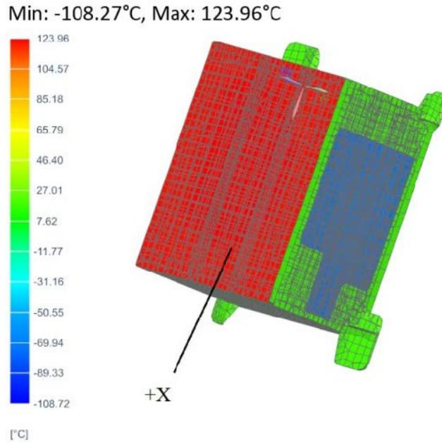
Figure 1.9: Thermal model of the "AIST" small satellite. Taken from Ivanushkin et al [ITS<sup>+</sup>19].
