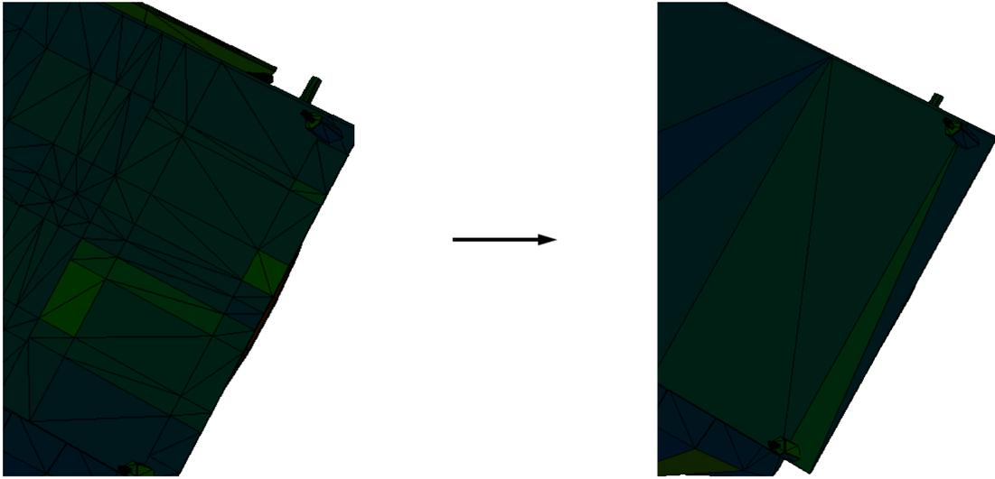
Figure 4.27: Closeup of a part hidden from direct fluxes before and after reduction with simulation without cluster constraints. Since the clusters depicted here (one color for each cluster) do not contribute to the considered simulation, they disappear during the reduction process.
