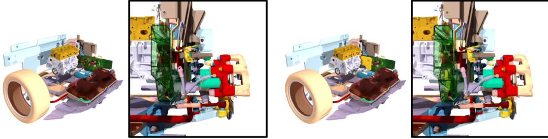
Figure 2.19: Multiple meshes decimation from Ghazanfarpour et al [GMH<sup>+</sup>20]. Left: 425 meshes and 3M faces. Right: 150k faces.
