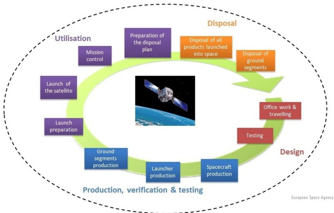
Figure 1.1: Life cycle of a satellite, from esa.int.
