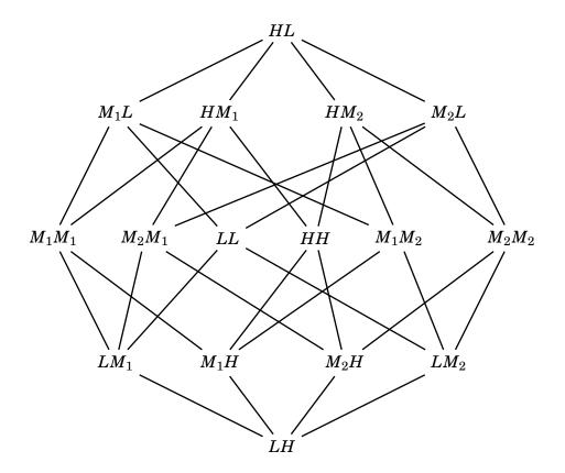
Figure 5.4: A diamond lattice of security levels.
