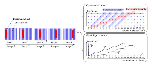
Figure 3.7: Graph construction example: the blue texture background has a disparity of 1 at each view and the red rectangle foreground has a disparity of 3 for each view. This example graph contains all different types of pixels: a) appearing, b) disoccluded, c) occluded and d) disappearing.
