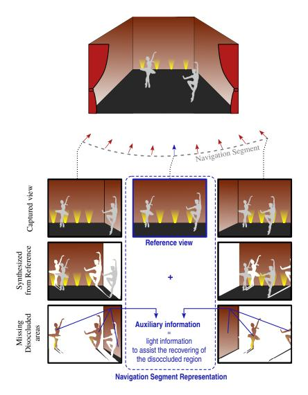
Figure 2.5: Proposed representation of a navigation segment: a reference view and an auxiliary information.
