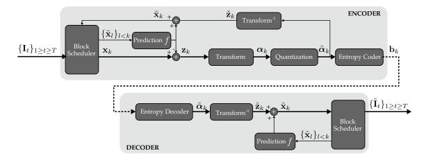
Figure 1.1: Structure of a conventional video encoder/decoder. The performance are measured by both the rate  $R = \sum_k |\mathbf{b}_k|$  and the distortion  $D = \sum_k ||\mathbf{x}_k - \tilde{\mathbf{x}}_k||_2^2$ .
