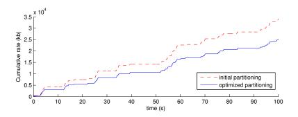
Figure 2.8: Cumulative rate computation during a user's navigation. Both navigation domain partitioning are compared: the *initial* one based on the camera distance only, and the optimized one, for which our method is adopted to adapt the size of the navigation segments to the scene content.
