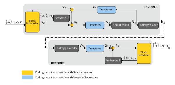
Figure 1.7: Limitations of conventional coding architecture.
