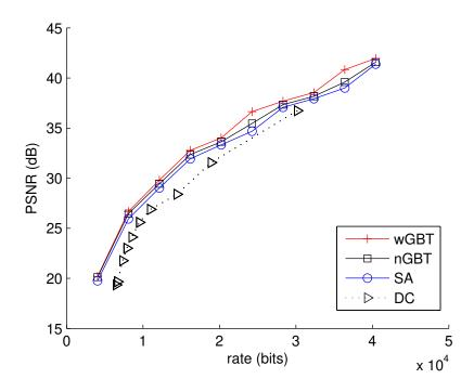
Figure 3.11: Rate-distortion evaluation for multi-view coding (geometry+luminance).
