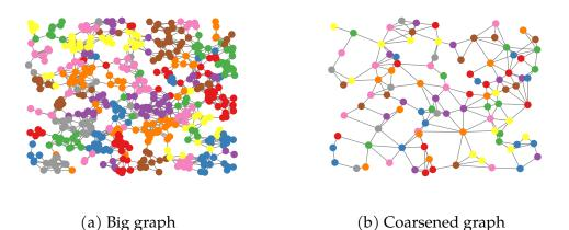
Figure 4.8: Illustration of coarsening result with [114]. Colors depicts the pixels that are merged during the coarsening process.
