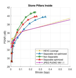
Figure 4.7: Example of Rate Distortion performance obtained with our graph based coding scheme (Non separable, not optimized and optimized separable graph transforms) compared to Light Field coding baselines.
