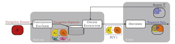
Figure 2.4: The navigation domain is partitioned into navigation segments, and each navigation segment is encoded and stored on a server. Users interact with the server to request the navigation segments needed for the navigation.
