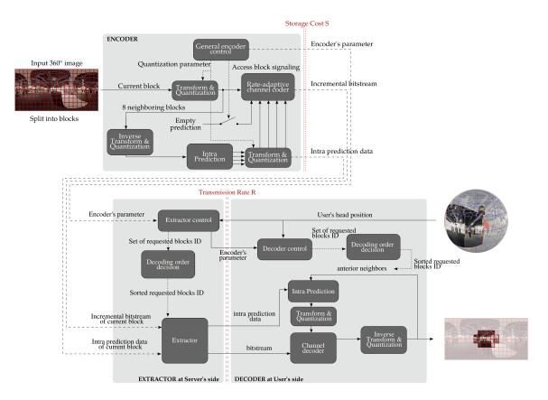
Figure 2.14: Proposed interactive coding scheme for omnidirectional data.
