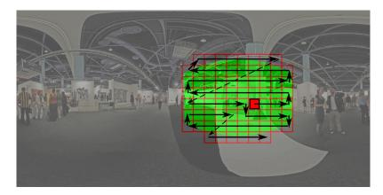
Figure 2.15: Decoding process. The red block is the access block. The arrows indicate the decoding order.
