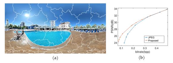
Figure 4.4: Rate-distortion optimized graph segmentation for 360°.
