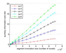
Figure 2.7: Illustration of the evolution of the size of auxiliary information  $R(\varphi_i)$  as a function of the number of voxels in the segment innovation. The auxiliary information is coded with a DCT-based scheme with uniform quantization of the coefficients, where q corresponds to the number of bits used to describe each DCT coefficient.
