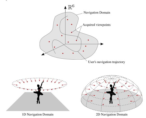
Figure 2.3: The navigation domain is a manifold included in  $\mathbb{R}^6$ , corresponding to the 6 degrees of freedom a user can play with during his navigation. The set of acquired views (in red) corresponds to a discrete set included in this navigation domain.
