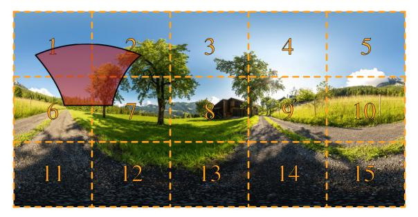
Figure 2.2: An omnidirectional image represented in equirectangular format and divided into 15 tiles. As an example, when the user's viewport corresponds to the red zone, the tiles 1, 2, 6 and 7 are transmitted instead of the whole image.
