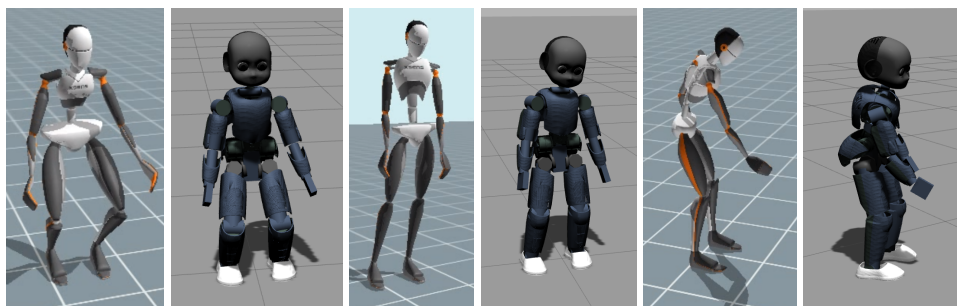
Figure 2.8: Snapshots of simulations of the teleoperated robot and of the Xsens skeleton while performing a squat motion, a hip roll exaggerate motion and a grasping motion.
