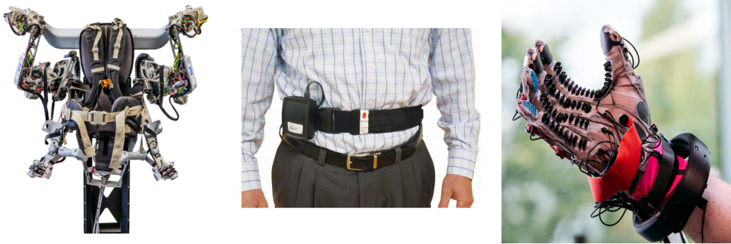
Figure 1.4: Examples of interfaces used to get haptic feedback from the robot. From left to right: exoskeleton (credits: DFKI), vibro-tactile belt (credits: Biodex) and haptic gloves (credits: Facebook Reality Labs)
