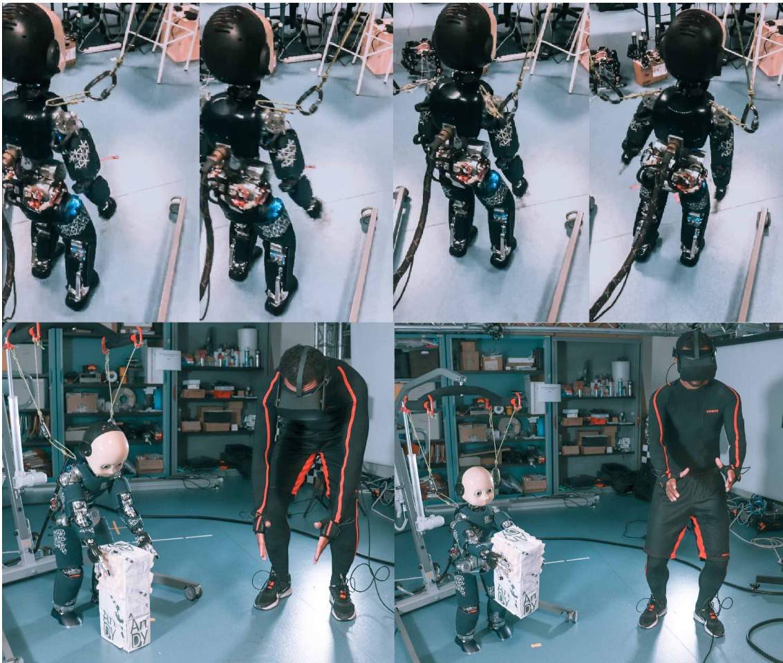
Figure 4.5: Snapshots from the teleoperation experiment with the iCub robot. Top: robot walking in the high-level mode. Bottom: robot controlled in the low-level mode with a motion capture suit and a VR headset.
