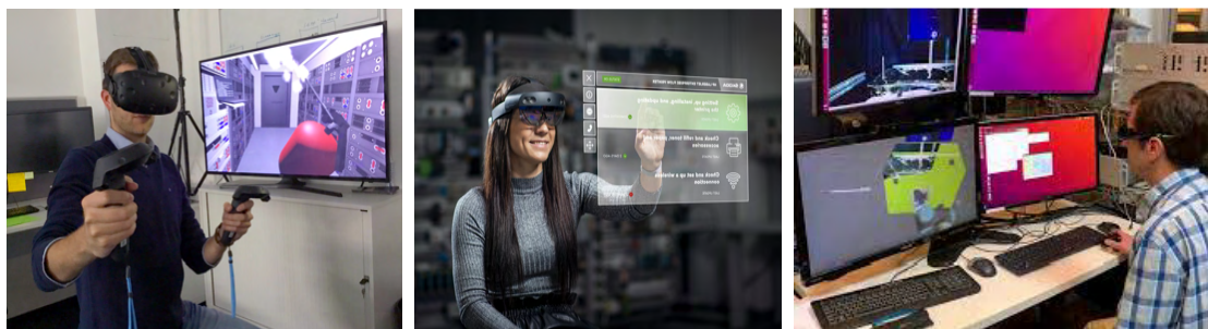
Figure 1.3: Examples of interfaces used to get visual feedback from the robot. From left to right: Virtual Reality headset (CC BY-SA 3.0 IGO), Augmented Reality headset (credits: ŠKODA AUTO a.s. 2022) and Graphical User Interface [93].
