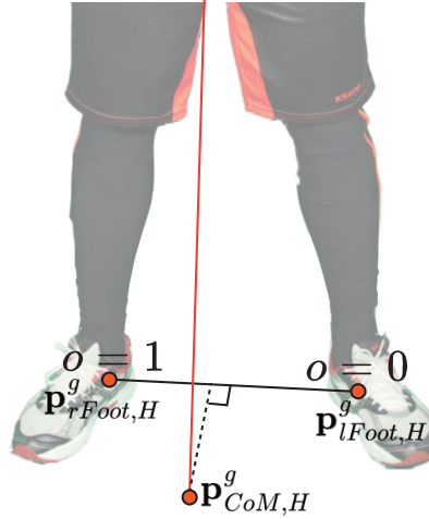
Figure 2.4: Normalized offset center of mass computation. The normalized offset is computed from the ground projection of the center of mass \mathbf{p}_{CoM,H}^g and the feet positions of the human.
