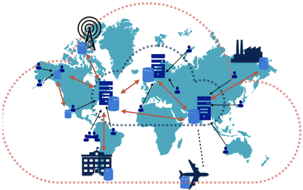
Fig. 2.2.: An example of the Edge Computing model. The cloud model presented in figure 2.1 is extended with new data replicas, closer to the users (i.e., the edge or the border of the network), this heterogeneous model mixes partial data replicas in a gigabyte wired school (high quality connections are illustrated with red arrows) or a manufacture company, a disconnected plane that will be reconnected after landing, users also store replicas in their own devices and can collaborate directly among them without the need to synchronize via the cloud server.
