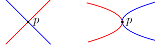
Figure 4.1: Left: At an A_1 singularity, two branches of the curve intersect transversally. Right: At an A_{2k+1} singularity with k > 1 , the tangent lines of the two branches at the intersection point coincide.
