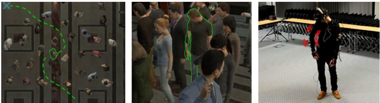
Figure 4.3: Our objective is to understand whether and to what extent providing haptic rendering of collisions during navigation through a virtual crowd (left) makes users behave more realistically [Berton et al. 2020a]. Whenever a collision occurs (center), armbands worn on the arms locally vibrate to render this contact (right). We carried out an experiment with 23 participants, testing both subjective and objective metrics regarding the user's path planning, body motion, kinetic energy, senses of presence and embodiment.
