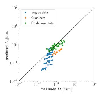
Figure 5.4: Predictions of the departure diameter correlation used in the MITB against experimental data.
