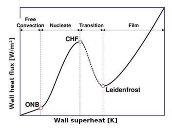
Figure 5.1: Nukiyama boiling curve, from [Liu et al., 2015].
