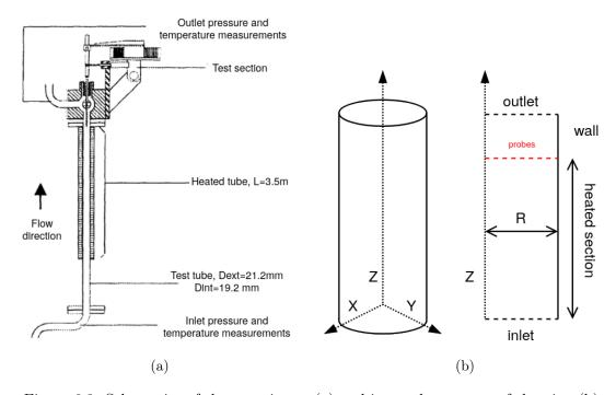
Figure 6.3: Schematics of the experiment (a) and internal geometry of the pipe (b).
