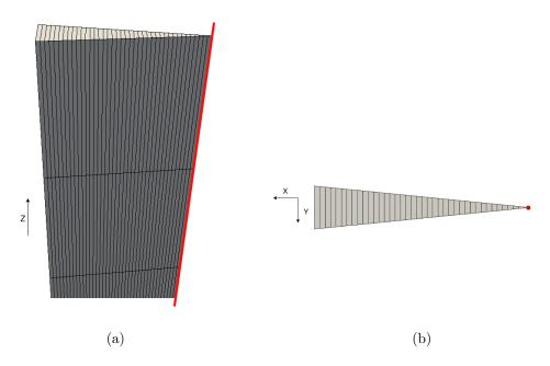
Figure 6.4: 3D axisymmetric mesh for the simulation of the A6 case, viewed from the side (a) and the top (b). The axis of symmetry is highlighted in red.
