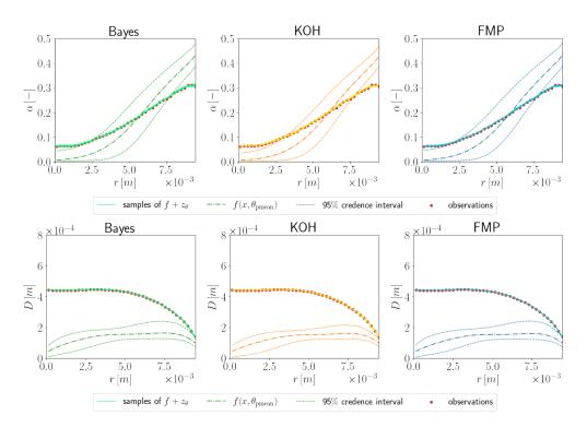
Figure 6.19: Predictions of void fraction (top row) and bubble diameter (bottom row), using void fraction and diameter observations. Note that the legend is the same for all figures on the same row, with color depending on the calibration method.
