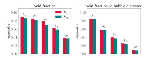
Figure 6.20: Ordered eigenvalues of the parameter posterior variance matrix (marginal and conditional), estimated from the Bayes sample, for both calibration studies. When the number of observations is higher (right figure), the posterior variance is smaller, corresponding to smaller eigenvalues with a faster decrease.
