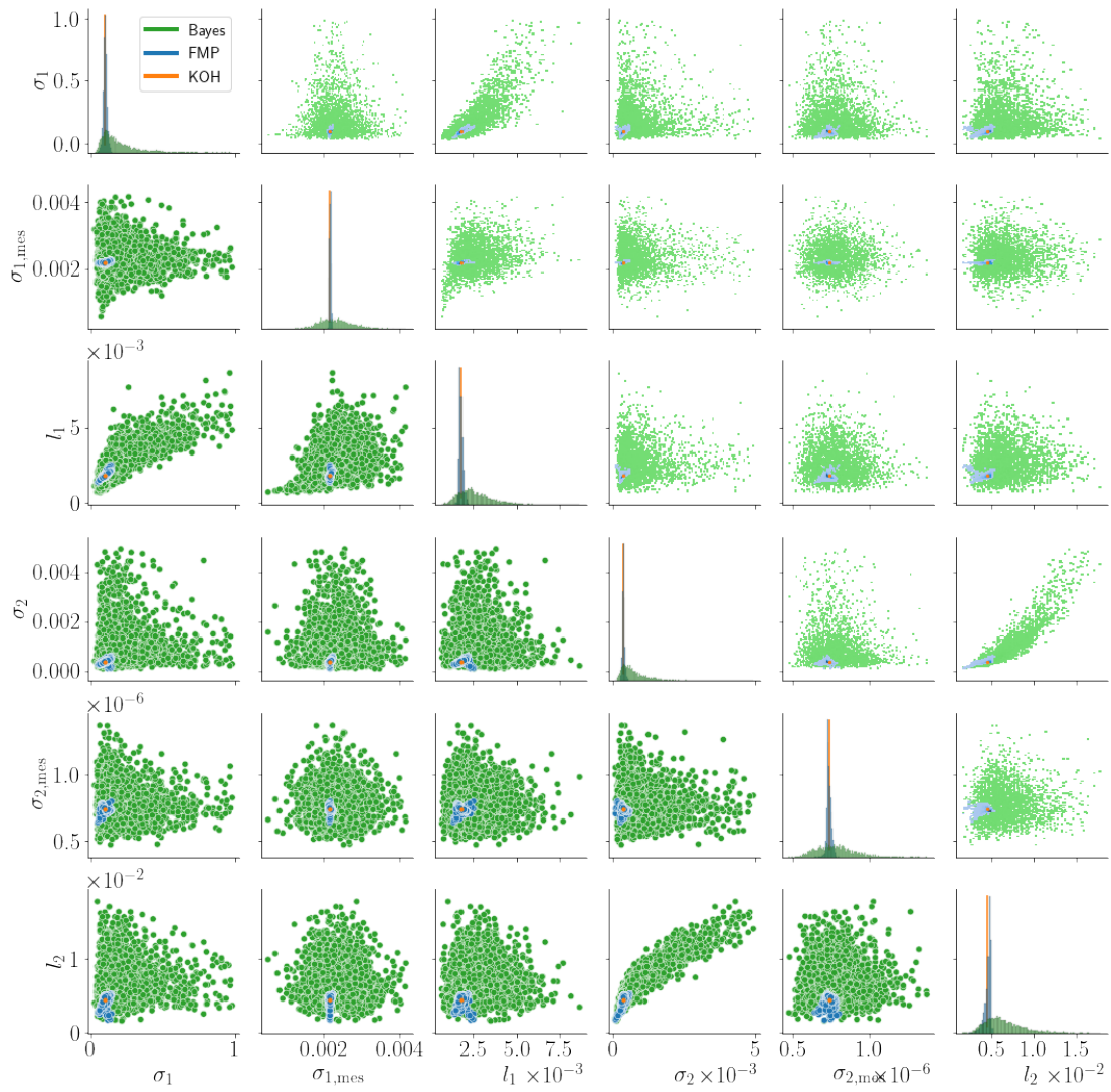
Figure 6.18: Posterior distribution of hyperparameters with the void fraction and bubble diameter observations.
