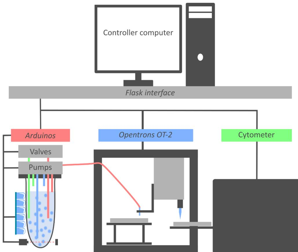
**Figure 3.4. Multi-bioreactors platform enabled for automated cytometry measurements and optogenetic control of continuous yeast cell cultures.** A unique controller computer orchestrates the platform function through the *Reacsight* strategy enabling full platform integration (Bertaux et al., 2021). The *Flask* API interfaces the different independent components of the platform and
