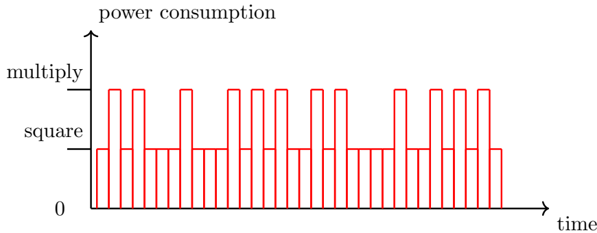
Figure 4.1: Power consumption analysis indicative example – square-and-multiply with exponent (1100100111011000101110)_2 . For clarity we use the exaggerated ratio of 2 : 1 for the power consumed by a multiplication, relative to a square.
