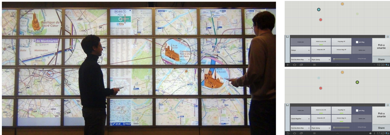
Figure 2.1: Smarties . On the left an example of a wall-display with multiple lenses on a map visualization (a magnification lens, a DragMag and a fisheye). Each analyst is holding a mobile tablet. On the right, the mobile client interfaces running on the tablets. In each tablet, the round colored pucks are attached to the position of the different lenses. The active puck is the blue one for the device on top, and the green for the bottom since each analyst is interacting with a different lens. The widgets added for this specific application are seen on the widget area at the bottom of the tablet interface.
