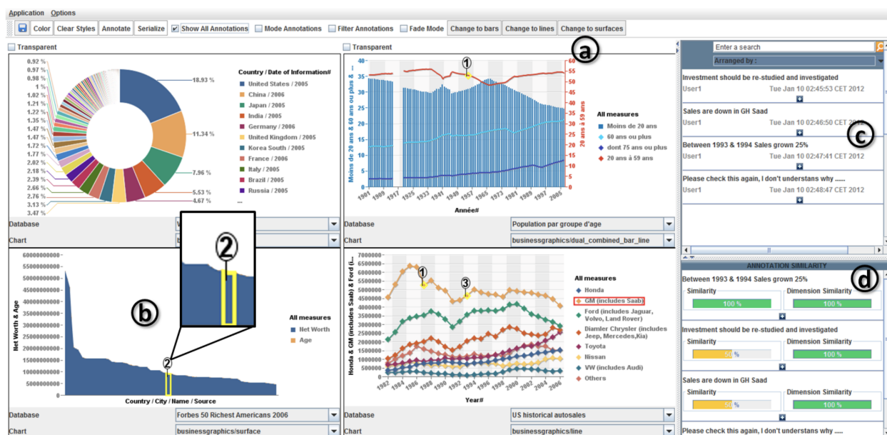
Figure 3.1: Context Aware Annotations. Our dashboard prototype with context aware annotations. (a) The main dashboard contains icons with the number of annotations for each data-point (b). Below the list of all dashboard annotations in (c), is a set of recommended annotations (d) emphasizing their similarity.
