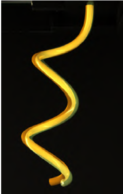
Fig. 1.3: Depiction of a simulated suspended rod over a physical physical one showing very good agreement. The simulation has been made using the exact known material parameters as that of the synthetically constructed physical rod.
