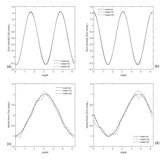
FIGURE 3.6 – Test case A. Reconstruction of the missing boundary data with noisy Dirichlet data over  $\Gamma_c$  with noise levels  $\sigma = \{1\%, 3\%\}$ . (a) exact and computed first components of the velocity over  $\Gamma_i$  (b) exact and computed second components of the velocity over  $\Gamma_i$  (c) exact and computed first components of the normal stress over  $\Gamma_i$  (d) exact and computed second components of the normal stress over  $\Gamma_i$ .
