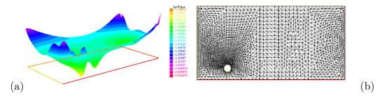
FIGURE 4.3 – Case A- Detection of a single object (for unnoisy data). (a) the iso-values of the topological gradient at convergence (b) the approximate location  $z_{opt}$  is equal to (-0.294, -0.174), while the exact one  $z_{ex}$  is equal to (-0.3, -0.15).
