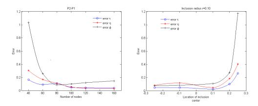
FIGURE 2.3 – Test case A. (Left) sensitivity of the reconstruction w.r.t. the mesh size (on abscissae : the number of F.E. nodes on the boundary  $\partial\Omega$ ). (Right) sensitivity of the reconstruction w.r.t. the distance to the inaccessible boundary  $\Gamma_i$  (on abscissae : the distance of the center of the circular inclusion from  $\Gamma_i$ ).
