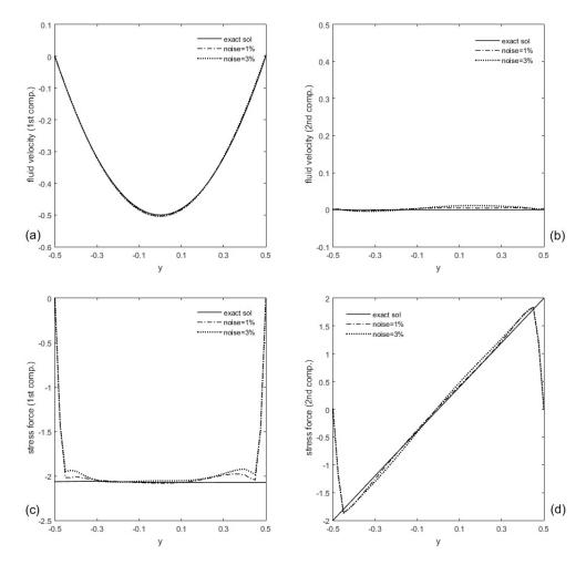
FIGURE 3.11 – Test case C. Reconstruction of the missing boundary data with noisy Dirichlet data over  $\Gamma_c$  with noise levels  $\sigma = \{1\%, 3\%\}$ . (a) exact and computed first components of the velocity over  $\Gamma_i$  (b) exact and computed second components of the velocity over  $\Gamma_i$  (c) exact and computed first components of the normal stress over  $\Gamma_i$  (d) exact and computed second components of the normal stress over  $\Gamma_i$ .
