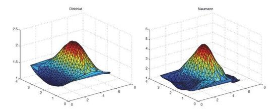
FIGURE 1.5 – Reconstructed nonradial Dirichlet ( $\tau_N$ , left) and Neumann ( $\eta_N$ , right) data over  $I_i$ . The profiles are presented at convergence and for a noise level  $\sigma = 5\%$  [56].
