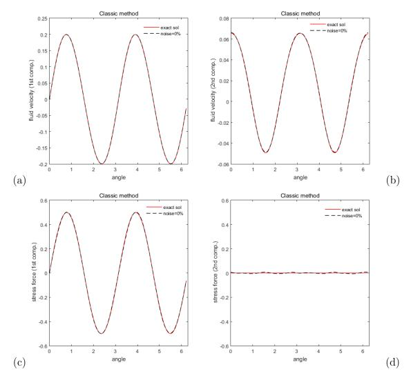
FIGURE 5.4 – Test case-A "Classic Method". Reconstruction of the missing boundary data from unnoisy data. (a) exact and computed first components of the velocity over  $\Gamma_i$  (b) exact and computed second components of the velocity over  $\Gamma_i$  (c) exact and computed first components of the normal stress over  $\Gamma_i$  (d) exact and computed second components of the normal stress over  $\Gamma_i$ .
