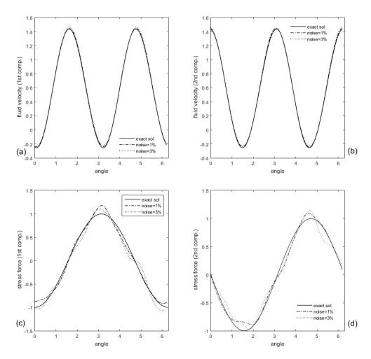
FIGURE 3.8 – Test case B. Reconstruction of the missing boundary data with noisy Dirichlet data over  $\Gamma_c$  with noise levels  $\sigma = \{1\%, 3\%\}$ . (a) exact and computed first components of the velocity over  $\Gamma_i$  (b) exact and computed second components of the velocity over  $\Gamma_i$  (c) exact and computed first components of the normal stress over  $\Gamma_i$  (d) exact and computed second components of the normal stress over  $\Gamma_i$ .
