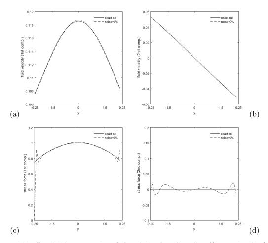
FIGURE 4.6 – Case B- Reconstruction of the missing boundary data (for unnoisy data). (a) exact -line- and computed -dashed line- first component of the velocity over  $\Gamma_i$  (b) exact -line- and computed -dashed line- second component of the velocity over  $\Gamma_i$  (c) exact -line- and computed -dashed line- first component of the normal stress over  $\Gamma_i$  (d) exact -line- and computed -dashed line- second component of the normal stress over  $\Gamma_i$ .
