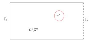
FIGURE 2.1 – An example of the geometric configuration of the problem : the whole domain including cavities is denoted by  $\Omega$ . It contains an inclusion  $\omega^*$ . The boundary of  $\Omega$  is composed of  $\Gamma_c$ , an accessible part where over-specified data are available, and an inaccessible part  $\Gamma_i$  where the data are missing.
