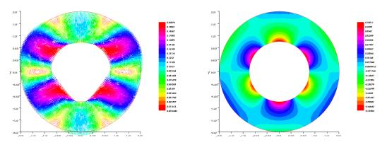
FIGURE 5.1 – Test case A. Iso-values of the velocity (left) and pressure (right) fields.
