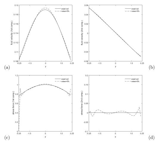
FIGURE 4.4 – Case A- Reconstruction of the missing boundary data (for unnoisy data). (a) exact -line- and computed -dashed line- first component of the velocity over  $\Gamma_i$  (b) exact -line- and computed -dashed line- second component of the velocity over  $\Gamma_i$  (c) exact -line- and computed -dashed line- first component of the normal stress over  $\Gamma_i$  (d) exact -line- and computed -dashed line- second component of the normal stress over  $\Gamma_i$ .
