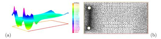
FIGURE 4.5 – Case B- Detection of two objects (for unnoisy data). (a) the iso-values of the topological gradient at convergence (b) the approximate locations are equal to  $z_{opt}^1 = (-0.422006, -0.160662)$  and  $z_{opt}^2 = (-0.416224, 0.159772)$ , while the exact ones are equal to  $z_{ex}^1 = (-0.4, -0.15)$  and  $z_{ex}^2 = (-0.4, 0.15)$ .
