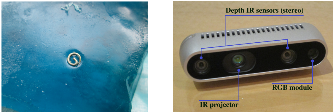
Figure 5.12: Left: Example of a laparoscopic tackers, which is generally used to attach artificial materials to the tissues. Right: Overview of an Intel RealSense D435 RGB-D camera. It has a color sensor to obtain an RGB image and an infrared (IR) projector with two IR sensors to reconstruct the scene depth.
