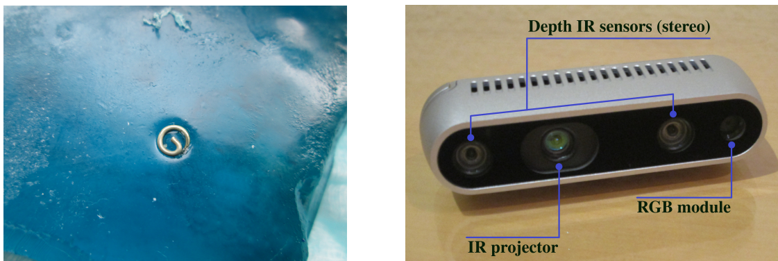
Figure 5.12: Left: Example of a laparoscopic tacker, which is generally used to attach artificial materials to the tissues. Right: Overview of an Intel RealSense D435 RGB-D camera. It has a color sensor to obtain an RGB image and an infrared (IR) projector with two IR sensors to reconstruct the scene depth.
