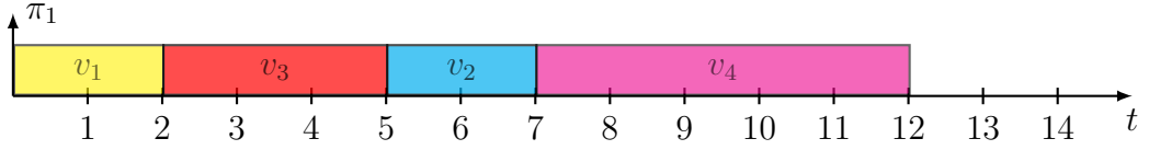
Figure A.2: Scheduling of DAG graph defined in Figure A.1 and Table A.1 according to the solution of MILP formulation with new constraints.
