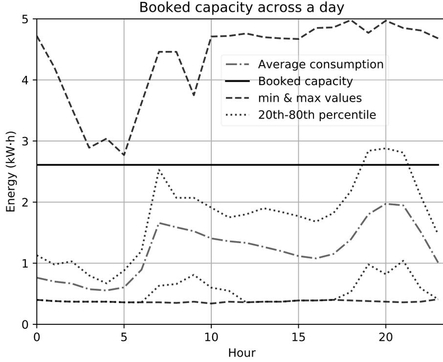
Figure 4.3 Booked capacity profile and load distribution bounds
