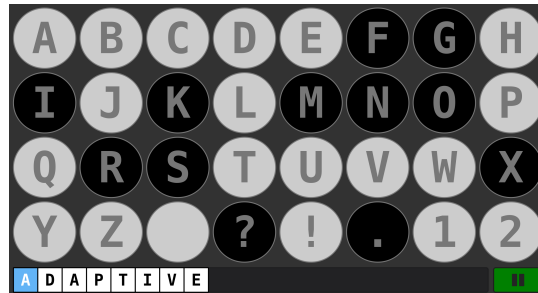
FIGURE 4.1 – Virtual keyboard developed for the c-VEP BCI system. During the stimulation the target is highlighted in blue below the keyboard.
