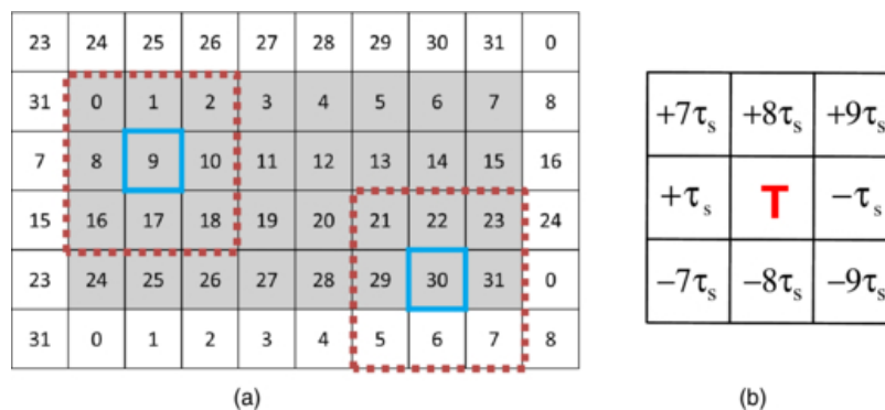
FIGURE 2.6 – The arrangement of the targets in the virtual keyboard following the principle of neighboring targets. Adapted from [Bin et al., 2011].
