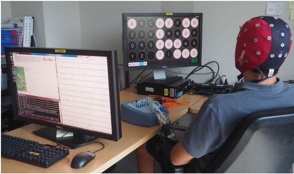
FIGURE 4.2 – Experimental setup. A subject wearing an EEG headset during the second phase of the experimental protocol. The subject is focusing his attention on the character highlighted in blue in the word written below the virtual keyboard. The other screen on the left is used to monitor in real time the subject’s EEG.
