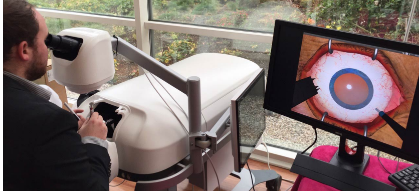
Figure 1.2: Retina surgery simulator with haptic feedback
