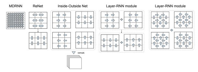
Figure 4.2 Schematic representation of the recurrent structure of different spatio-temporal recurrent models.
