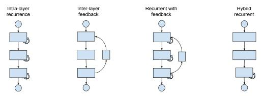
**Figure 4.1** Proposed taxonomy of recurrent and feedback CNN architectures. Each family is represented by an archetypal small module of 3-4 layers. Top and bottom circles stand for module's input and output, respectively.
