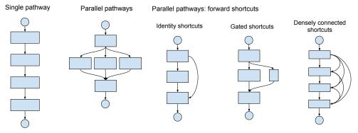
**Figure 3.1** Proposed taxonomy of feedforward CNN architectures. Each family is represented by an archetypal small module of 3-4 layers. Top and bottom circles stand for module's input and output, respectively.
