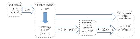
**Figure 6.1** The three layer model. The input data is fed to a convolution neural network, transforming the original image into a set of feature vectors. Then the information in this high dimensional feature space is summarized via a set of prototypes, in order to understand the landscape. Finally, the relation between a given data point and the label to infer is calculated through their proximity to the prototypes.
