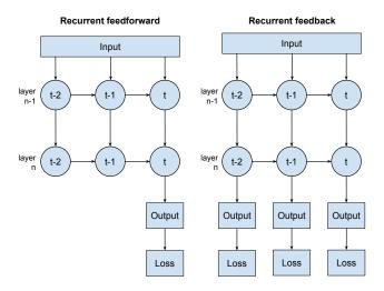
**Figure 4.3** Feedback nets predict an output at every time-step, connecting the loss to intermediate hidden states and changing how features are learned. Adapted from Zamir et al (2017).
