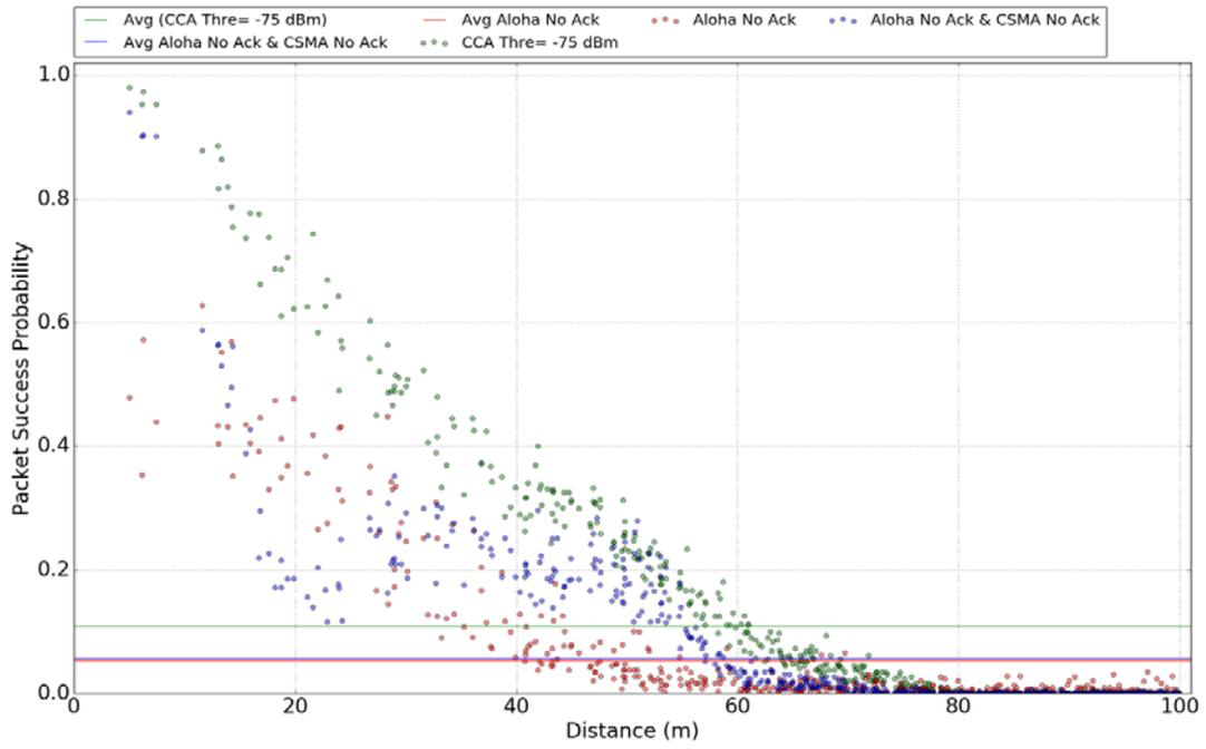
Figure 6.4 : Node PSP and distance to gateway for heterogeneous networks.
