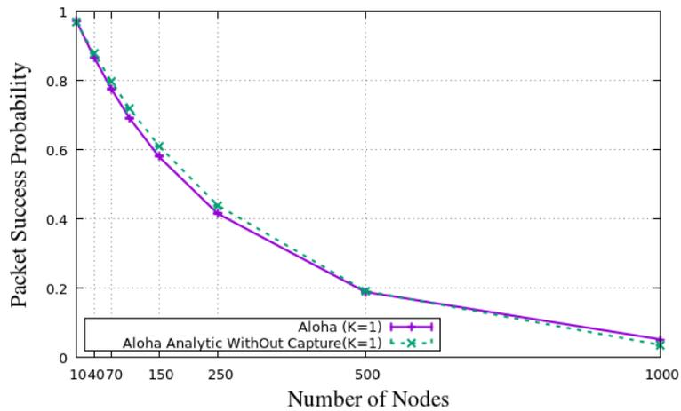
Figure 4.1 : Analytical model and simulation results when  $K=1$
