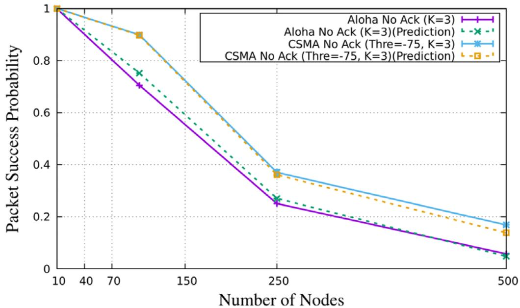
Figure 6.7 : Simulation results vs CNN prediction results
