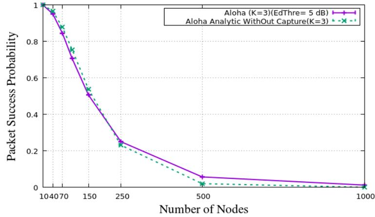
Figure 4.3 : Analytical model and simulation results when  $K=3$
