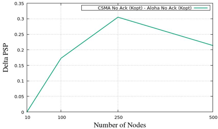
Figure 5.17 : PSP gain obtained by CSMA No Ack with respect to Aloha No Ack
