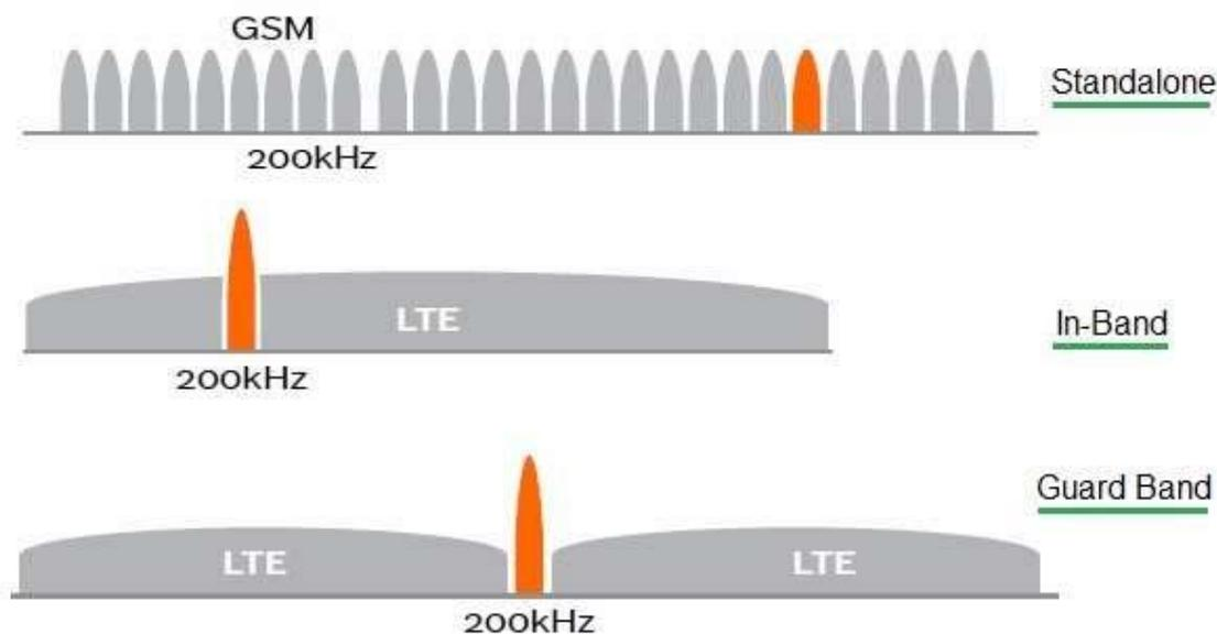
Figure 2.6: Frequency spectrums supported by NB-IoT [85]
