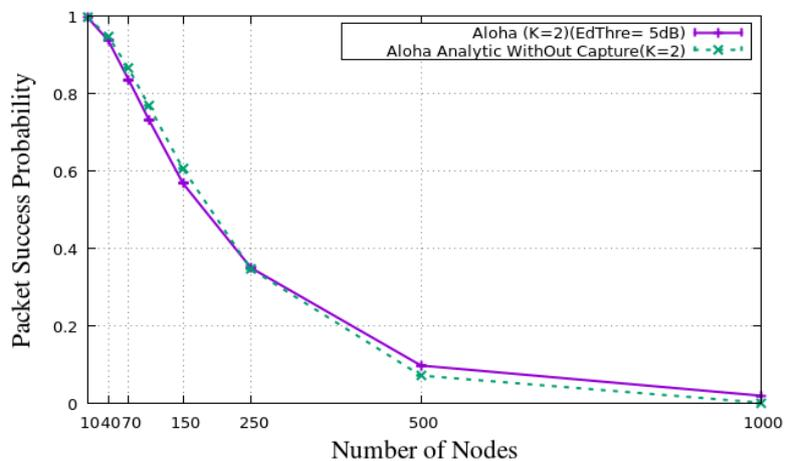
Figure 4.2 : Analytical model and simulation results when  $K=2$
