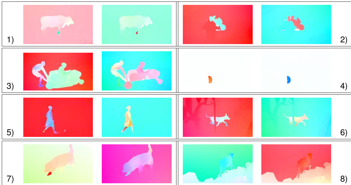
FIGURE 4.5 – a) Optical flows computed between two successive images of the videos illustrated in Figure 4.4. The backward element is on the left and the forward on the right for each sample.
