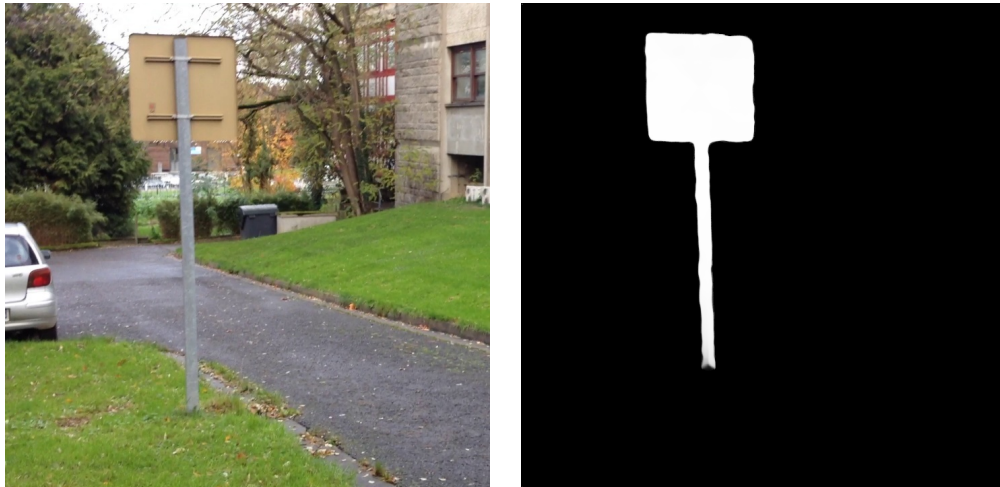
FIGURE 4.16 – Valued motion saliency map in presence of depth discontinuity in the scene. The traffic sign stands in the foreground, and consequently, has a different apparent motion (larger motion) due to the moving camera than the rest of the static background. Accordingly, it is found salient by MSI-ns, while it is a static object. Note that this frame is classified as not salient by the motion saliency detector presented in Chapter 3.
