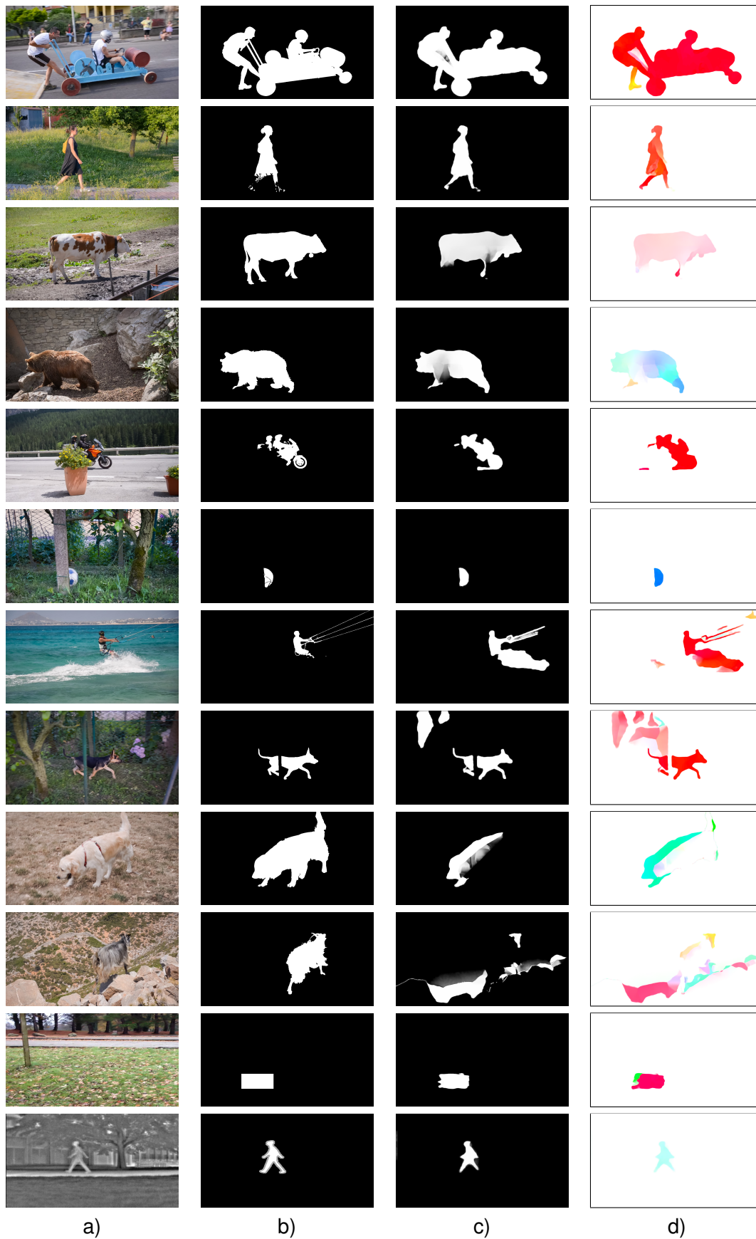
FIGURE 4.15 – From left to right : a) one image from the video, b) binary ground truth, c) motion saliency maps predicted by our method MSI-ns, and d) the estimated forward residual flow (displayed with the motion colour code of Figure 4.2).
