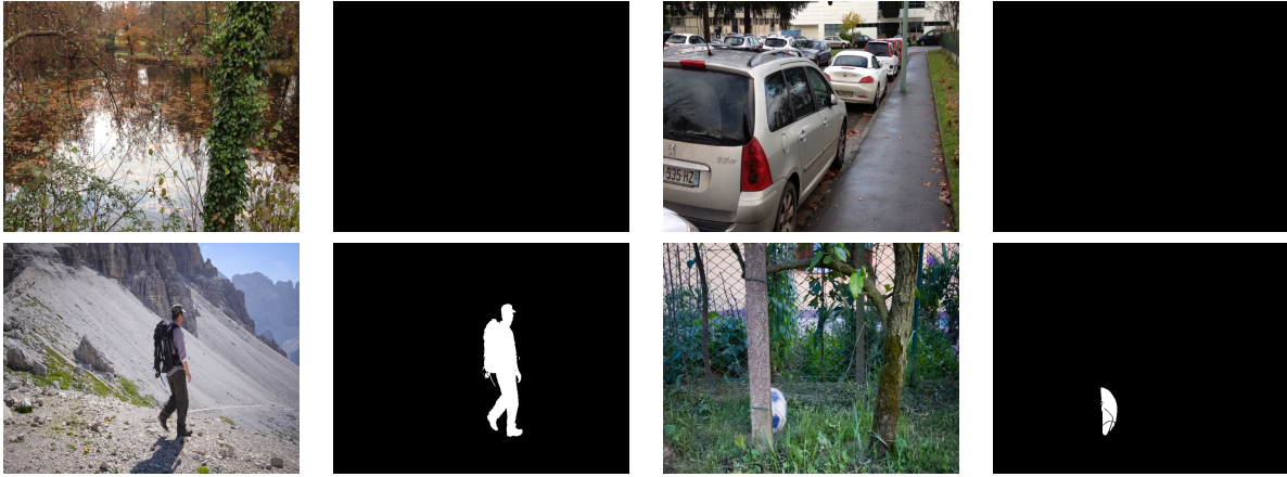
FIGURE 1.2 – Ground-truth motion saliency maps associated to four examples. A first possibility is that no element of the scene undergoes any salient motion. In this case, we get an empty ground truth saliency map. The two first samples correspond to such a situation. We acquired these videos as part of the dataset described in Chapter 3. In contrast, salient moving elements are present in the two last samples, as highlighted in the ground truth. The two last samples come from the DAVIS 2016 dataset [Per+16].
