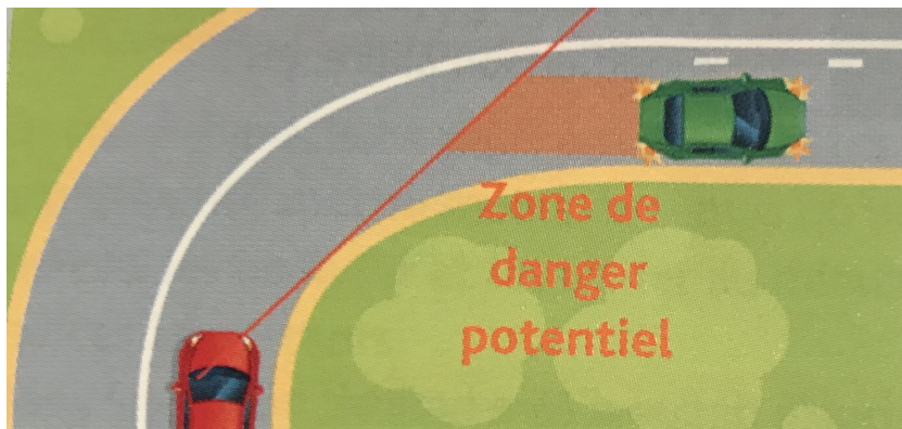
(a) “Area of potential danger”. A partial observability stemming from sensor occlusion in a turn.
