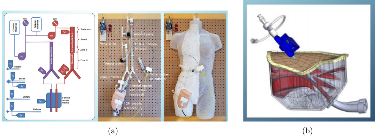
Figure 6.3: (a) Set-Up of the ER-REBOA simulator. (b) Render of the external sensor for catheter insertion tracking.
