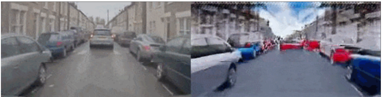
Figure 2.22 (a) Process flow of an end-to-end system for training and deployment, (b) images used by the network to decide with real perceived images (left) and the image transferred into the simulation space, after [101]
