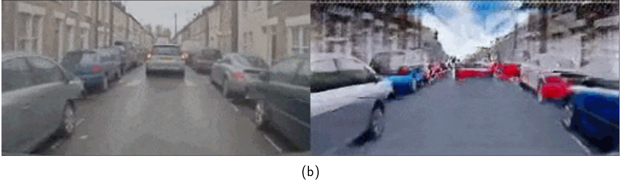
Figure 2.22 (a) Process flow of an end-to-end system for training and deployment, (b) images used by the network to decide with real perceived images (left) and the image transferred into the simulation space, after [101]
