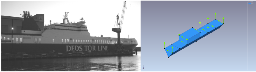
Figure 3.12: The ferry at the Flensburg shipyard (left). The geometry of the ferry with 16 acceleration channels attached (right).
