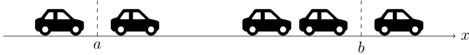
Figure 1.1 – Conservation of the number of vehicles on an unidirectional stretch of road.
