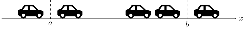
Figure 1.1 – Conservation of the number of vehicles on an unidirectional stretch of road.
