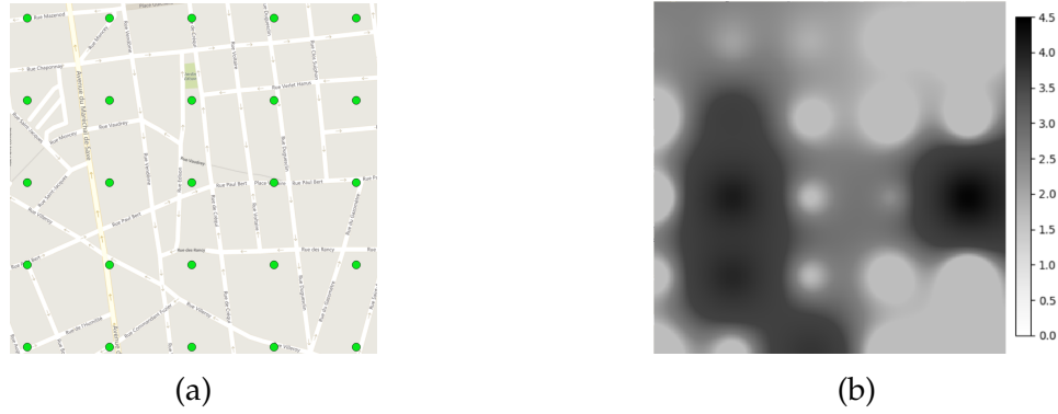
Figure 6.6: WSN nodes' locations and simulation errors' variance ( \mu g^2/m^6 ) corresponding to the district of La-Part-Dieu during June 2008.
