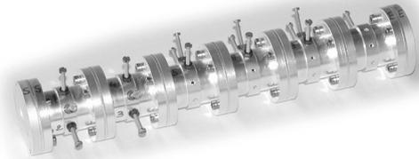
Fig. 8. Realized 11-pole four-zero asymmetrical dual-band bandpass filter.
