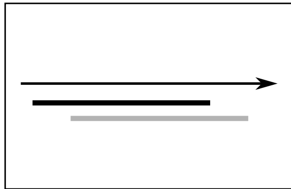
Figure 4.2.4 – Runtime Stacking Configuration: Temporal Concurrent. The black and grey are both running at the same time during a time period.
