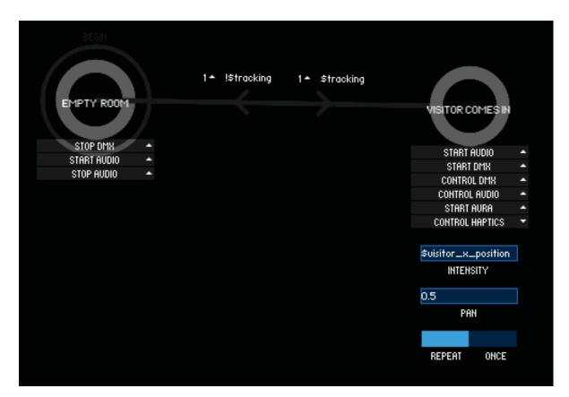
**Fig. 5.1** ZenStates allows users to quickly prototype interactive environments by directly manipulating *States* connected together via logical *Transitions. Tasks* add concrete actions to states and can be fine-tuned via high-level parameters (e.g. 'intensity' and 'pan'). *Blackboard* global variables (prefixed with the '\$' sign) can enrich tasks and transitions. (C) 2018 IEEE.
