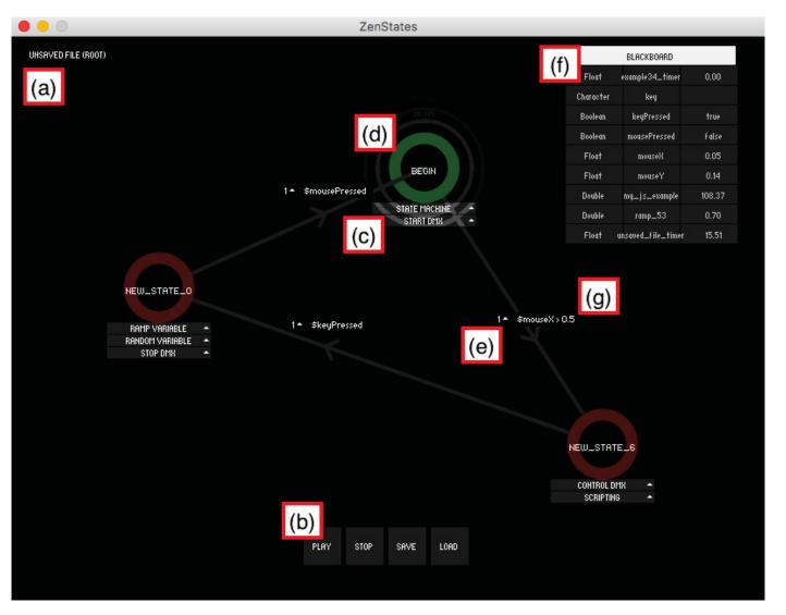
**Fig. 4.6** ZenStates' interface: (a) the state machine name; (b) control buttons; (c) tasks associated to a state; (d) the initial state (in this case, also the one which is currently running, represented in green); (e) a transition priority; (f) the blackboard; and (g) a transition.
