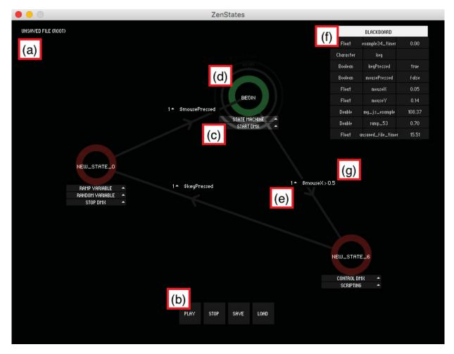
**Fig. 5.2** ZenStates' components: (a) the state machine name; (b) control buttons; (c) tasks associated with a state; (d) the initial state (in this case, also the one which is currently running, represented in green); (f) the blackboard; and transitions, composed by a guard condition (g) and its execution priority (e). (C) 2018 IEEE.
