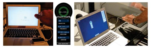
Fig. 6.6 We can quickly modify our theremin example to make it more realistic (image (c)) in two steps. First, we use the Leap Motion sensor and an OSC converter software (image(a)). Second, we modify our previous example from Figure 6.3 to match image (b): that is, we replace 'mouseX' and 'mouseY' variables by the incoming-OSC blackboard variables ('left\_hand\_z\_0' and 'right\_hand\_z\_0') and add a note augmenter to eliminate the need of key pressings.
