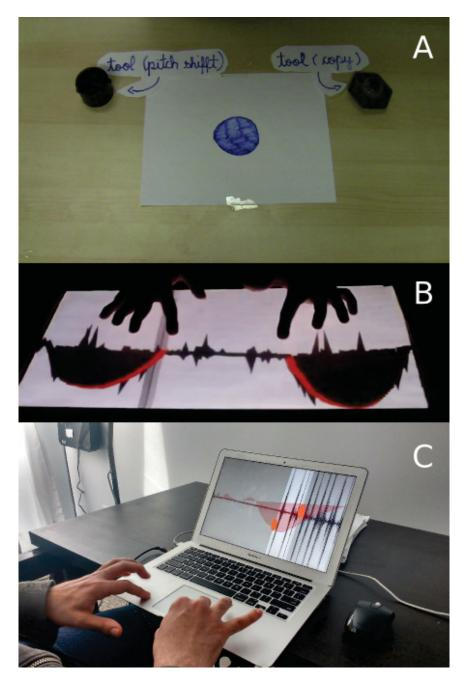
**Fig. 3.2** Several prototypes were designed for exploring our guidelines. In addition to paper sketches, we also built (A) a video prototype; (B) a functional prototype using a DIY multitouch table; and (C) another functional prototype using the computer's trackpad.
