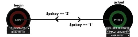
Fig. 6.5 Example of an interactive musical tool where users can switch between two different presets. When the user presses '1' on the computers' keyboard, presets described on state 'SYNTH 1' are loaded. On opposition, presets of 'SYNTH 2' state are loaded when '2' is pressed.
