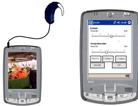
Figure 14.9 – A sampling software has been developed on a PDA that the patient plugs directly onto the CI processor in order to sample the exact sound that is received by the processor.
