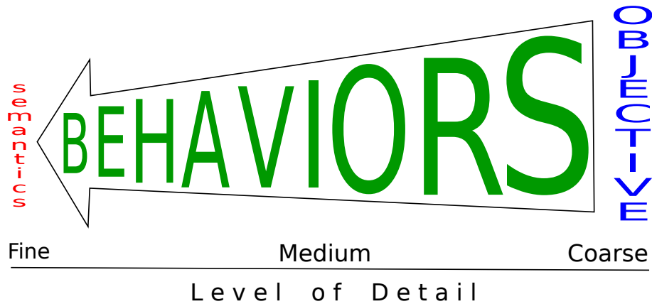
Figure 5.3 – Conceptual view of how the performance of a program can be analyzed. At one extreme we have objective-based analysis, a coarse view of performance. Semantics lies at another extreme, where a high level of detail is sought. Finally, behavior analysis provides a variable scale based on how the problem context is considered.
