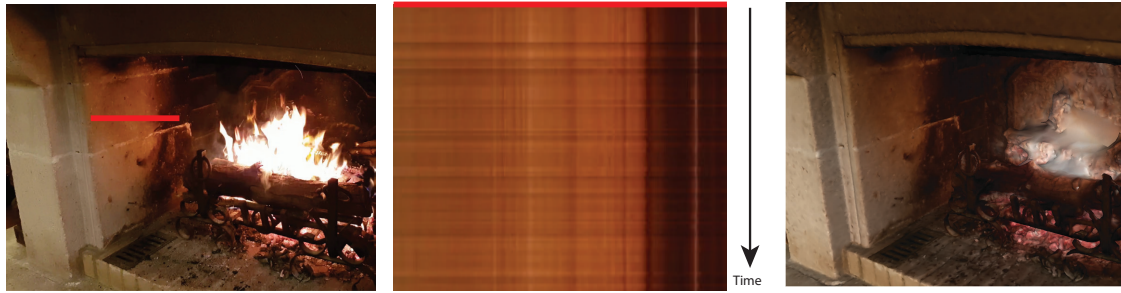
Figure 5.11: Time-dependent background. The dynamic flames indirectly change the appearance of the static background (horizontal patterns in the middle slice). However, they can be reprojected in novel views in a time-dependent manner onto the reconstructed geometry (colored mesh, far right).
