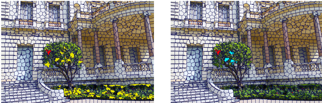
Figure 2.6: Super-pixel over-segmentation. To hallucinate depth in poorly reconstructed regions, Chaurasia et al. [21] use over-segmentation to propagate depth information. To create a reliable depth for the red super-pixel, 3 matches (cyan) are selected from a set of similar and close candidates (yellow).
