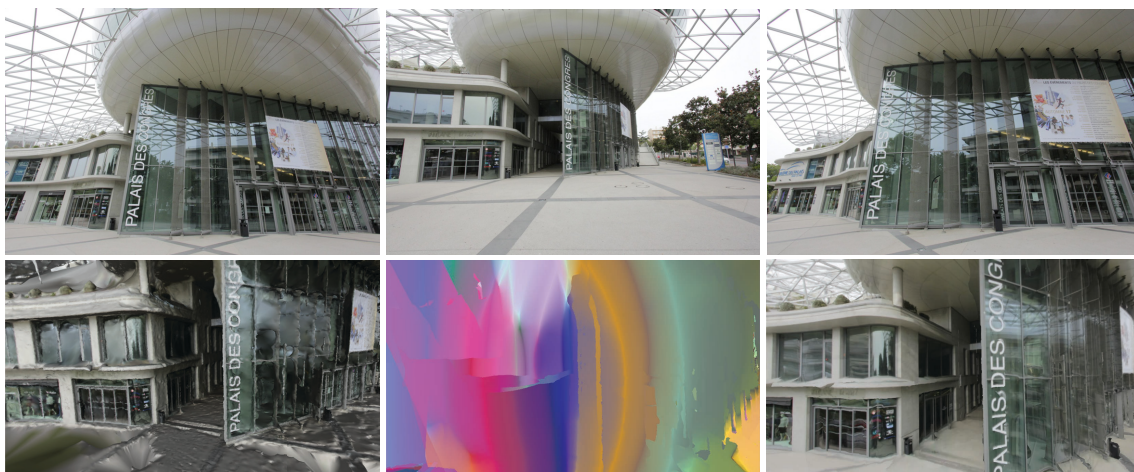
Figure 2.5: Reprojection Based IBR . From a set of wide-baseline captured images (top: 3 out of 50 input images), MVS methods are able to produce approximate geometry in a preprocessing step (bottom left). At runtime, the geometry is used to compute the contribution of each input image thanks to a blending obtained from the method of Buehler et al. [14] (middle bottom: a color is associated to each input camera). The input images are reprojected onto the geometry and blended accordingly, producing the final result (bottom right).
