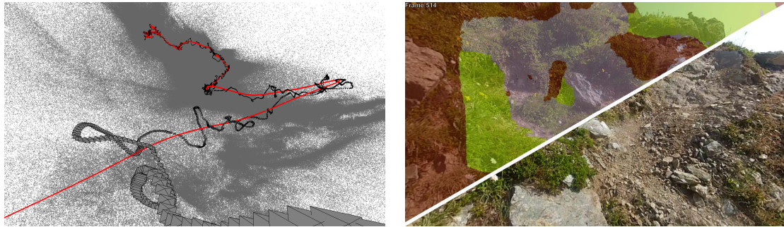
Figure 2.8: Hyperlapse . In order to stabilize video shots, Kopf et al. [63] find a suitable camera path for the novel view (left). To produce the final renderings, input video frames are stitched and blended using an offline global optimization (right).
