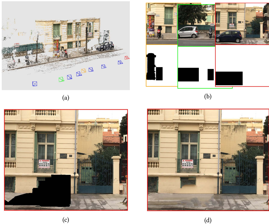
Figure 3.1: Method overview. (a) 3D reconstruction from multi-view input image dataset (b) Input images above, input masks below (c) Result of reprojection and mincut, remaining black pixels will be filled through patch-based inpainting (d) Inpainted result.
