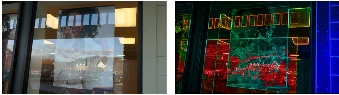
Figure 2.7: Gradient Domain IBR . By estimating depth at strong image edges, the method of Kopf et al. [64] reprojects image gradients from both real objects and objects reflected by planar surfaces.
