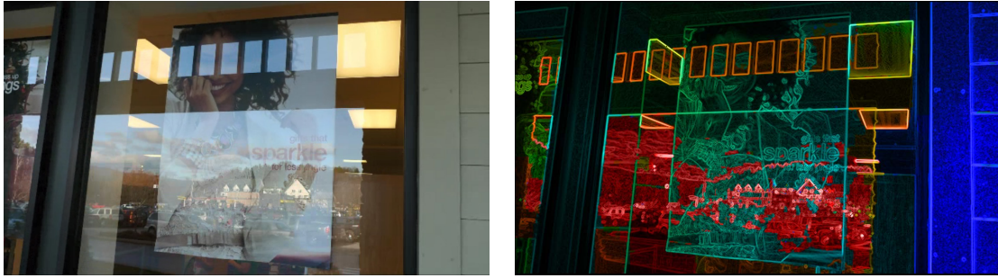
Figure 2.7: Gradient Domain IBR . By estimating depth at strong image edges, the method of Kopf et al. [64] reprojects image gradients from both real objects and objects reflected by planar surfaces.
