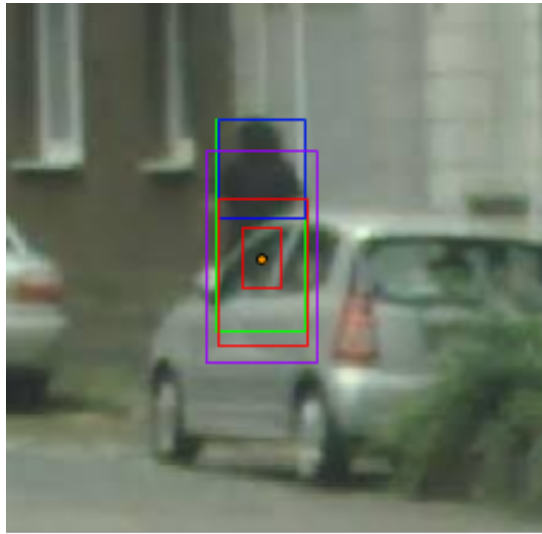
Figure 6.4: An occluded pedestrian with full-body bounding box ( green ) and visible bounding box ( blue ). Red anchors are confocal with the magenta anchor. The red anchors do not overlap well with both the full-body and visible bounding box, while the magenta anchor has sufficient overlap with both.
