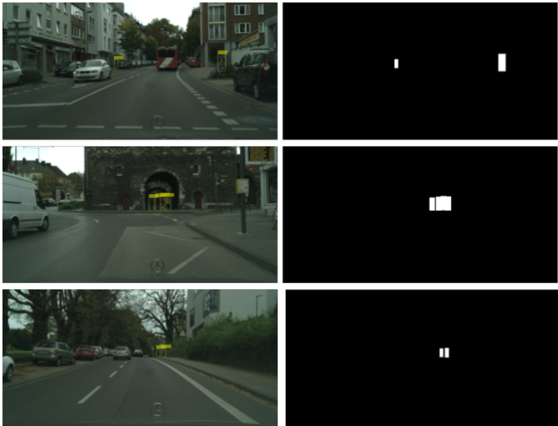
Figure 5.3: Left : An image with pedestrian bounding boxes. Right : The pseudo segmentation mask for the image on the left.
