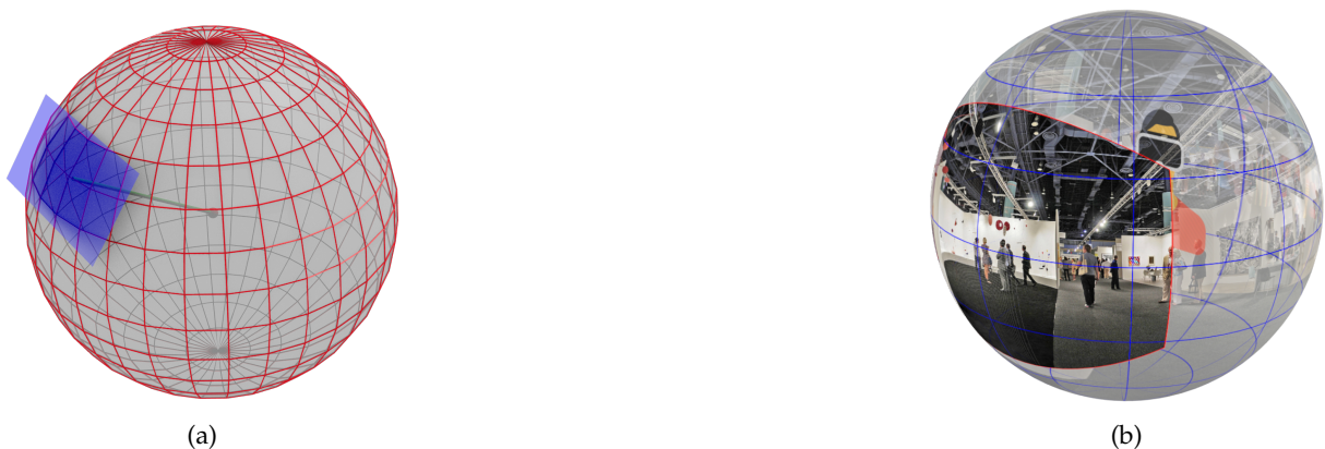
Figure 1.14 – Viewport requested from a 360° visual content. (a) An example of a viewport (in blue) requested by the user. The viewport plane is tangent to the sphere at the viewport center. The user direction is shown with a green line inside the sphere (from the sphere center to the viewport center). (b) An example of a portion corresponds to a request of full HD viewport with FOV of 110°. A request of the viewport corresponds to a small portion of the spherical content.
