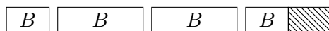
Figure 3.6: Representation of a solution for the 2DG-CSP-L corresponding to a batch B . The first plate has a smaller width, since it is the leftover from the previous batch. The right-hand part of the last plate will be re-used in the next batch.
