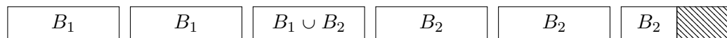
(a) Infeasible solution since it is not allowed to mix items from different batches in a cutting pattern
