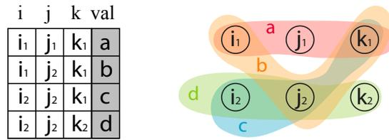
Figure 8.2: A sparse tensor and the associated hypergraph.
