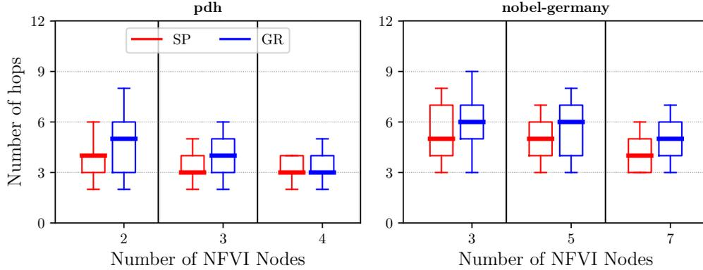
Figure 4.5: Hops distribution of the backup paths computed by the global rerouting schema (GR) compared with the shortest paths (SP) for `pdh` and `nobel-germany` networks. Boxes are defined by the first and third quartiles. Ends of the whiskers correspond to the first and ninth deciles.
