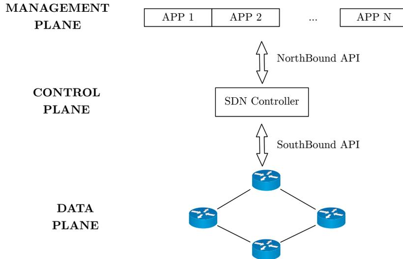
Figure 1.2: SDN Architecture with the interactions between layers
