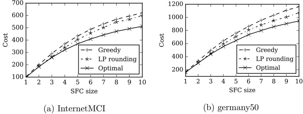
Figure 3.7: Average setup cost with respect to the length of the service function chains
