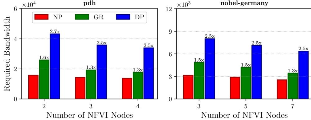
Figure 4.4: Bandwidth overhead comparison of the global rerouting (GR) and Dedicated Path Protection (DP) schemas with respect to the no-protection scenario (NP) for `pdh` and `nobel-germany` networks. Labels on top of the bars indicate the overhead with respect to the unprotected case.
