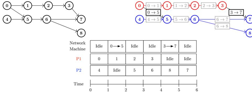
Figure 8.1: (Top Left) The dependency (di)graph of a job  $J$  with 9 (CPU) tasks. (Top Right) Modeling with network tasks indicated with rectangles. We provide a feasible schedule of job  $J$ . (Middle) Scheduled graph: (CPU) tasks executed by Machine 1 are in red, by Machine 2 in blue, carried out network tasks in black, not executed ones in gray. (Bottom) Timeline.
