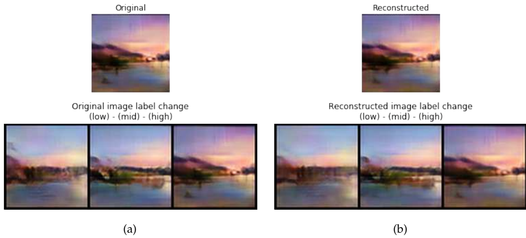
Figure 7.14: Latent vector search and label change for an image present in the generator space. The image reconstructed from the latent vector highly resembles original image, and the effect of the label change is also similar.
