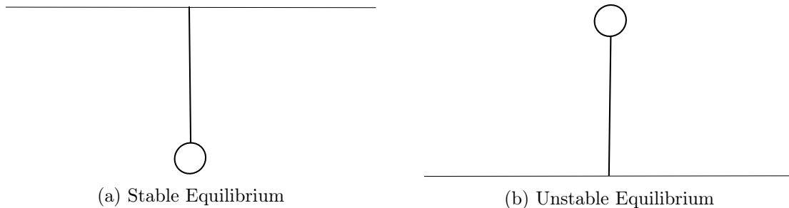
Figure 1.1 – The Two Equilibria of the Free Pendulum
