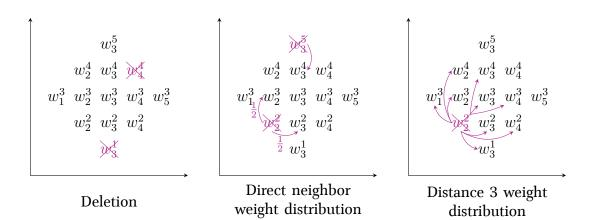
Figure 5.1 – Stencil Narrowing Strategies Reducing the number of computation of a stencil by reducing the number of points. The available strategies are: (1) deletion as presented on the left or (2) redistribution of stencil weights through direct neighbors (center) or up to a given distance (right).
