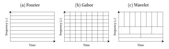
Figure 6.2 – Fourier, Gabor and Wavelet transformation time-frequency correlation
